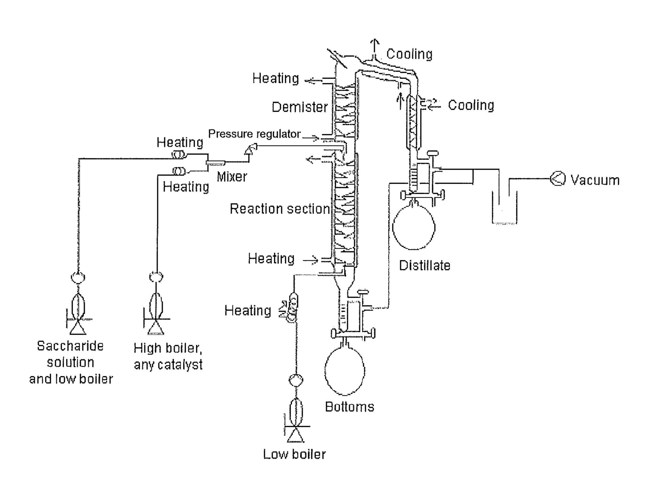
PREPARATION OF 5-HYDROXYMETHYLFURFURAL (HMF) FROM SACCHARIDE SOLUTIONS IN THE PRESENCE OF A SOLVENT HAVING A BOILING POINT GREATER THAN 60° C. AND LESS THAN 200° C. (AT STANDARD PRESSURE, CALLED LOW BOILER FOR SHORT)
