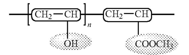
In certain embodiments polyvinyl alcohol (PVA) is a synthetic resin produced by polymerisation of vinyl acetate
