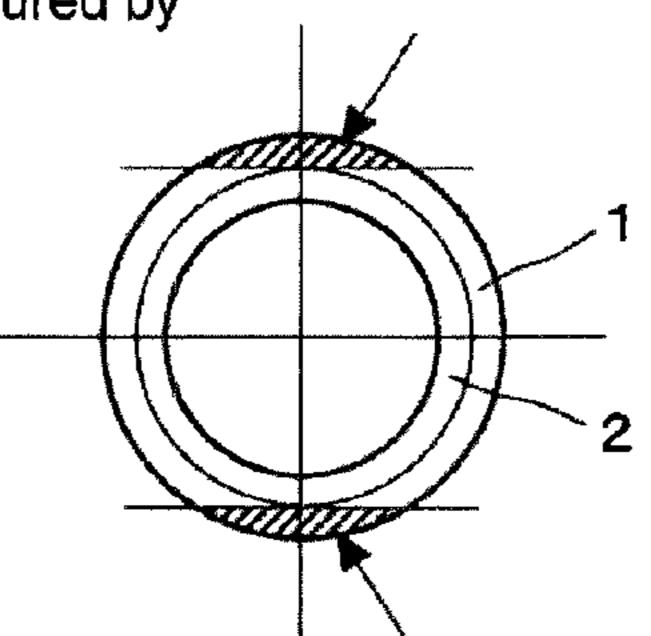
Portion of outer tube to be removed
