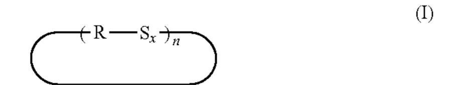
wherein R is a substituted or unsubstituted alkylene group having 4 to 8 carbon atoms, or a substituted or unsubstituted oxyalkylene group having 4 to 8 carbon atoms, x is 3 to 5 on the average, and n is an integer of 1 to 5.
