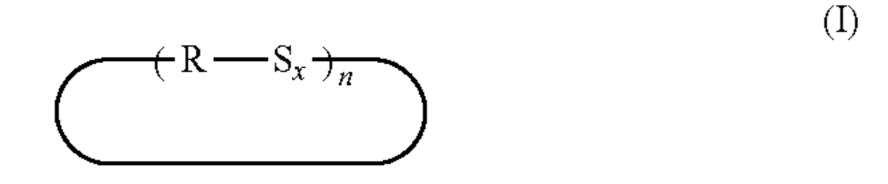
In the formula (I), R is a substituted or unsubstituted alkylene group having 4 to 8 carbon atoms, or a substituted or unsubstituted oxyalkylene group having 4 to 8 carbon atoms, x is 3 to 5 on the average, and n is an integer of 1 to 5.
