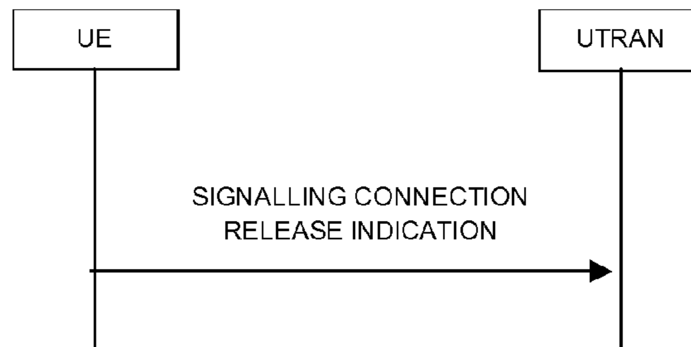
Figure 8.1.14-1: Signalling connection release indication procedure, normal case
