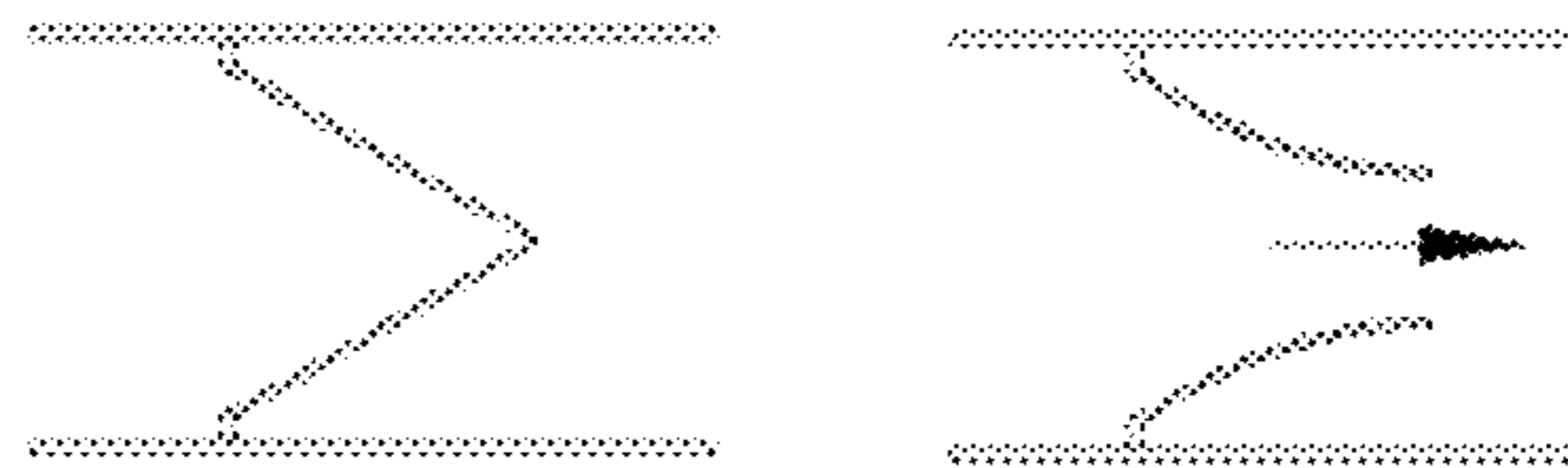
Reed Valve left: close right: open
