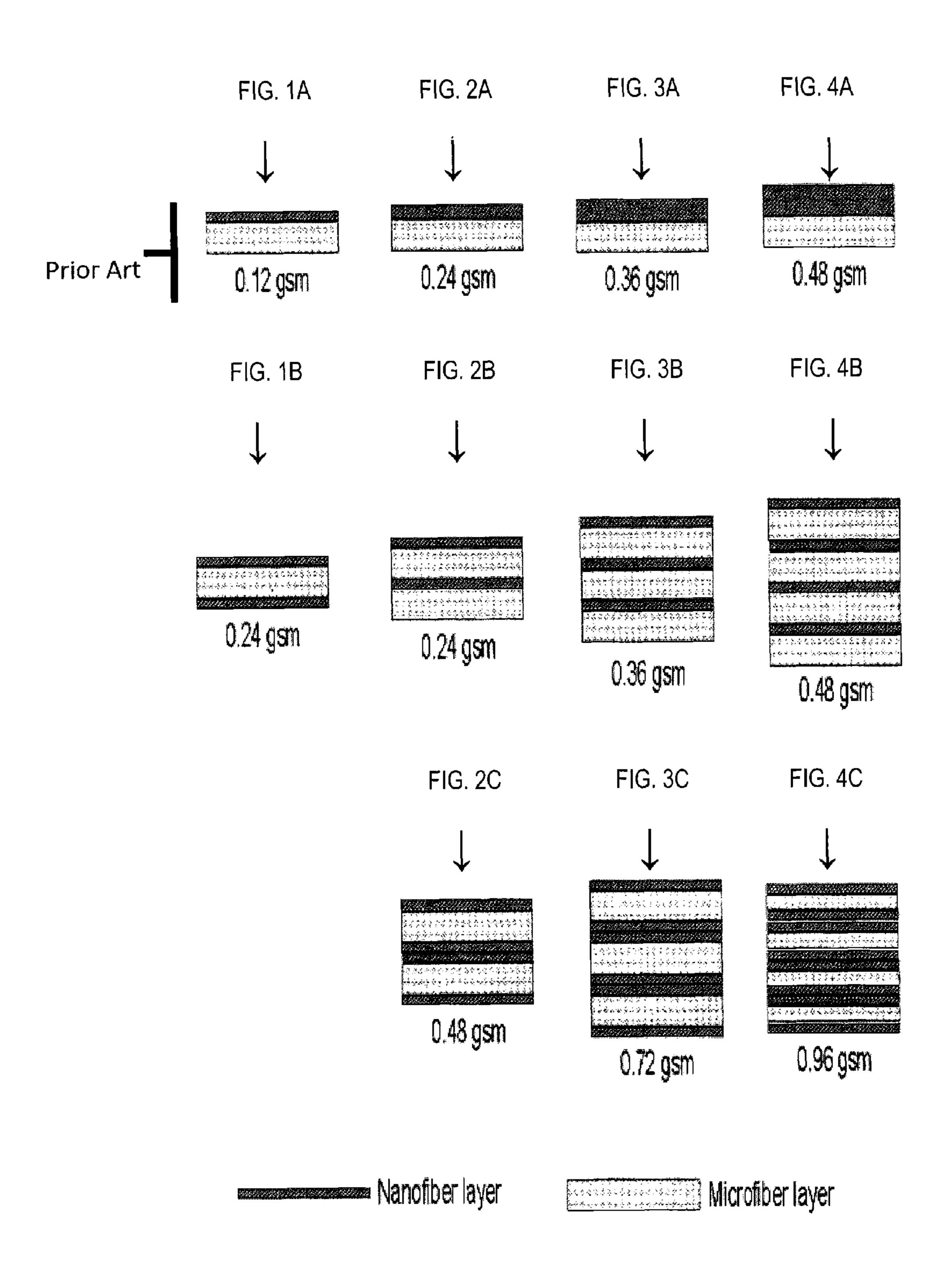
Thickness of nanofiber layer in different filtration medium as depicted in FIGs 1 to 4
