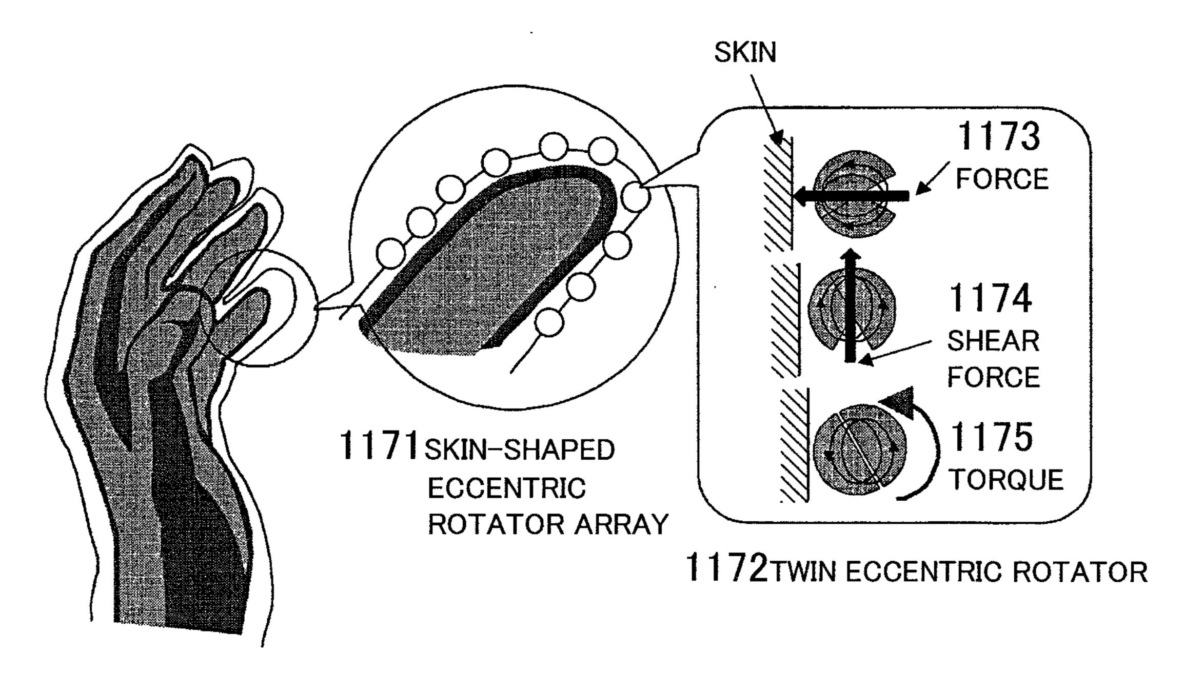
1170GLOVE-SHAPED ECCENTRIC ROTATOR ARRAY
