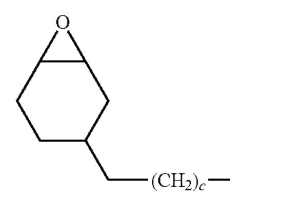
in which R<sup>2</sup> is an alkyl group, preferably a methyl group, or a hydrogen atom, ideally a hydrogen atom, a and c are integers ranging from 1 to 6, and b is 0, 1 or 2.
