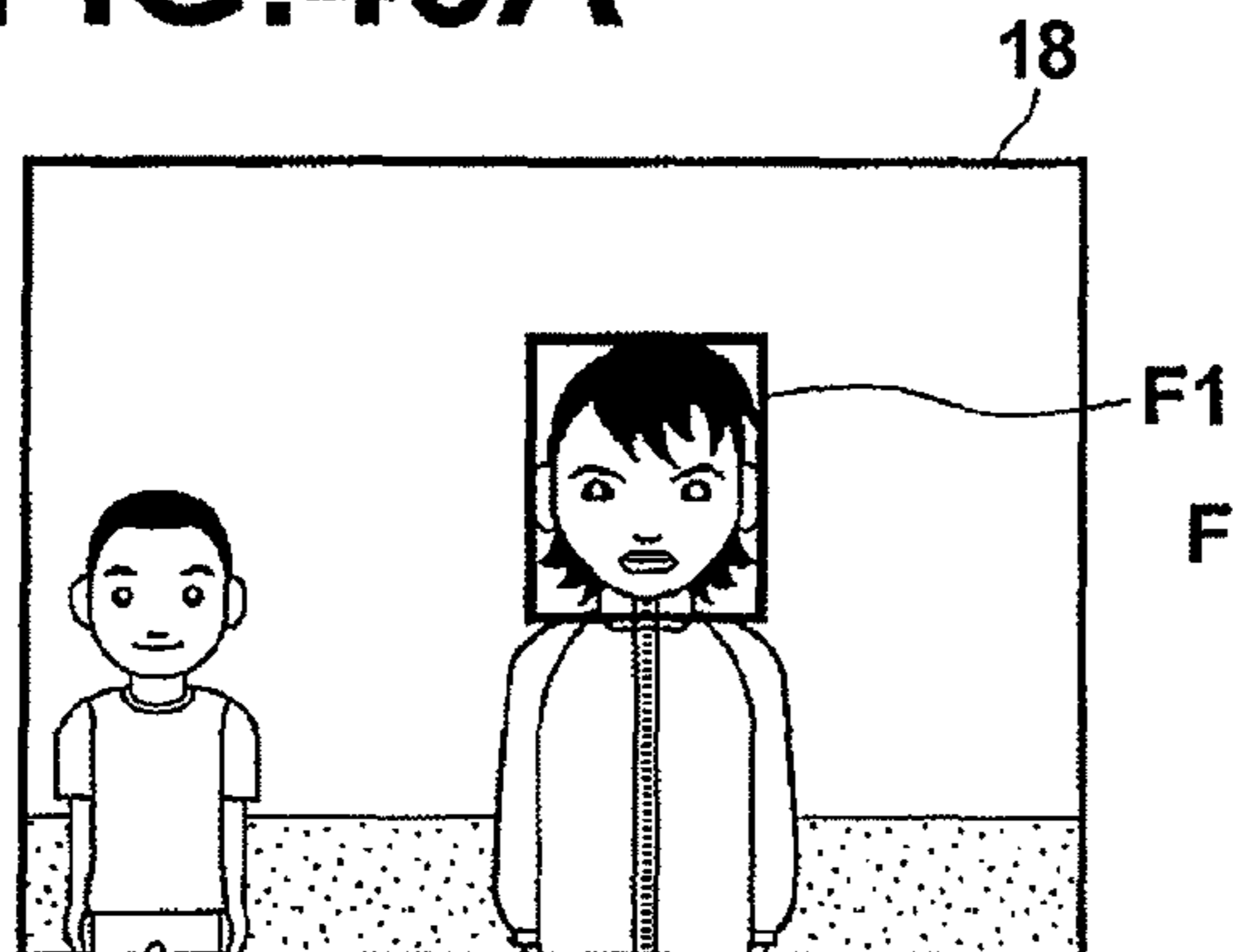
RESULT OF FACE DETECTION UNDER SETTING DURING PHOTOGRAPHING OPERATION
