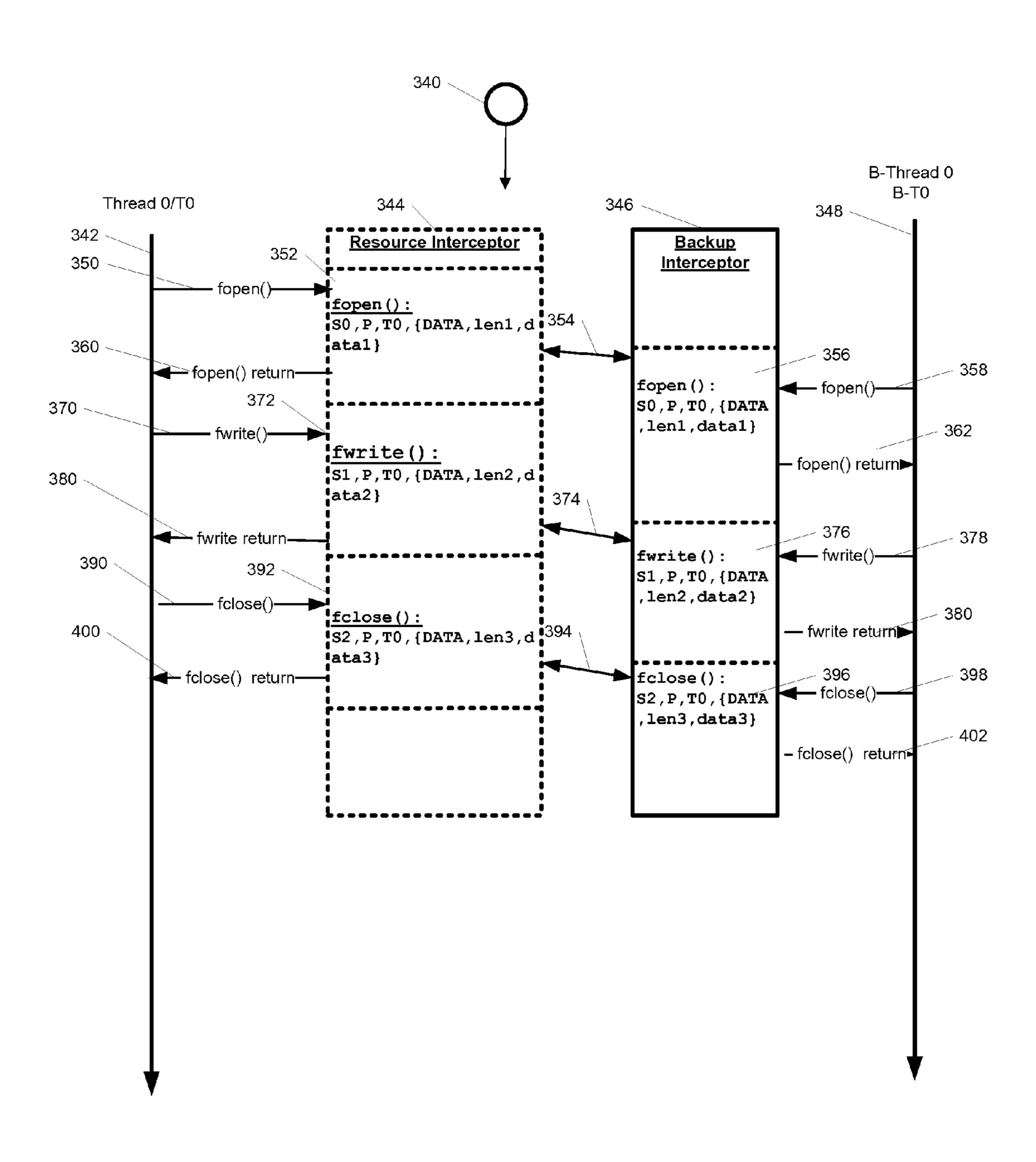
FIG.9 - I/O write processing
