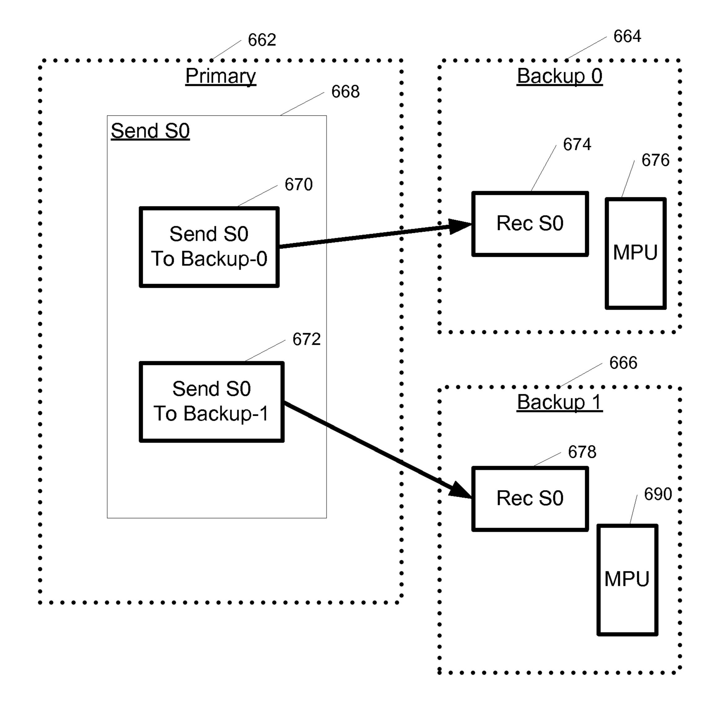
Fig.16 – Reliable messaging over TCP
