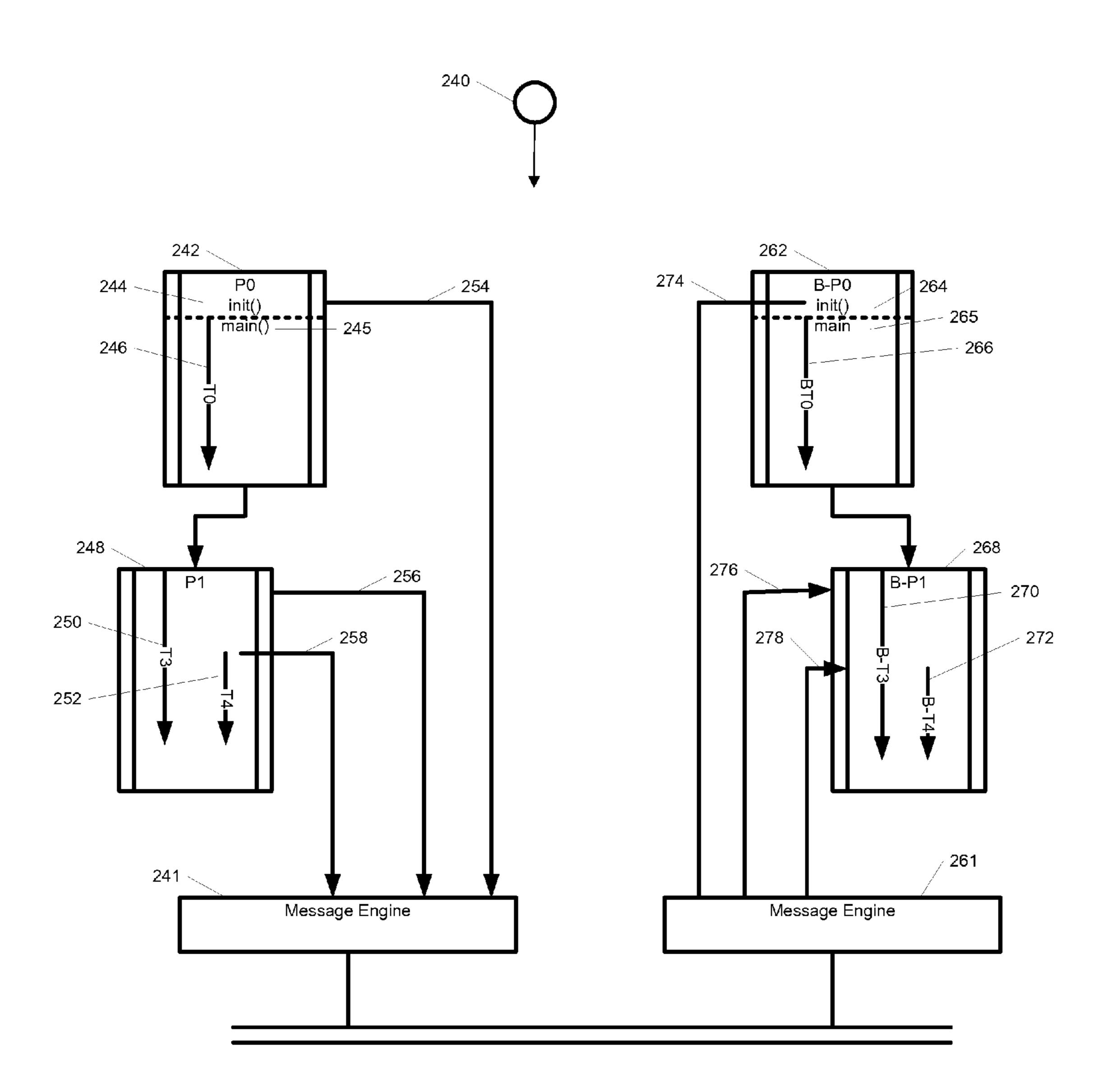
FIG.7 - Handling PROCESS messages
