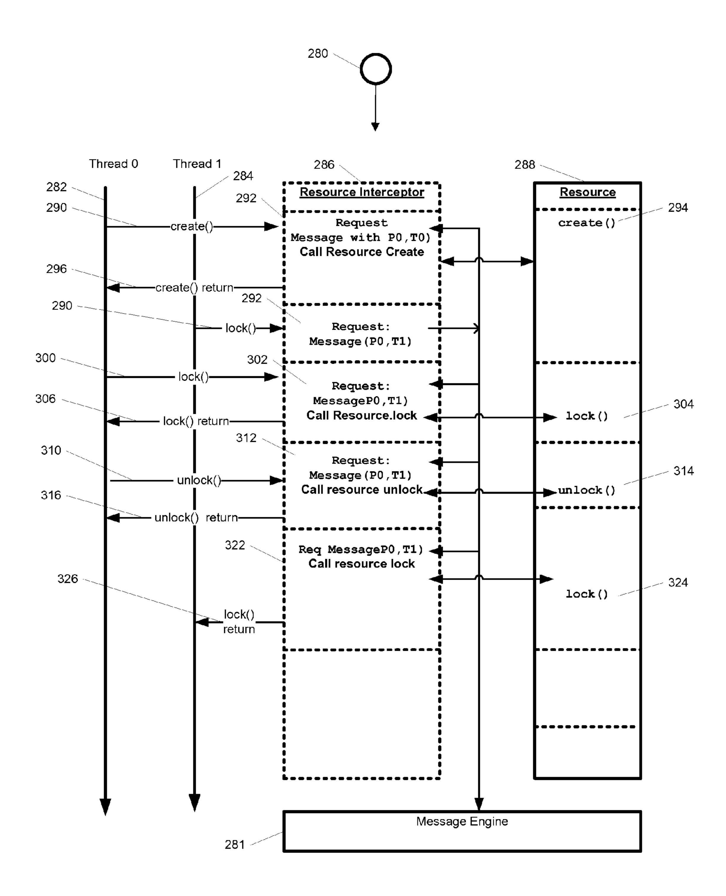
FIG.8 - Backup's Processing of replication messages
