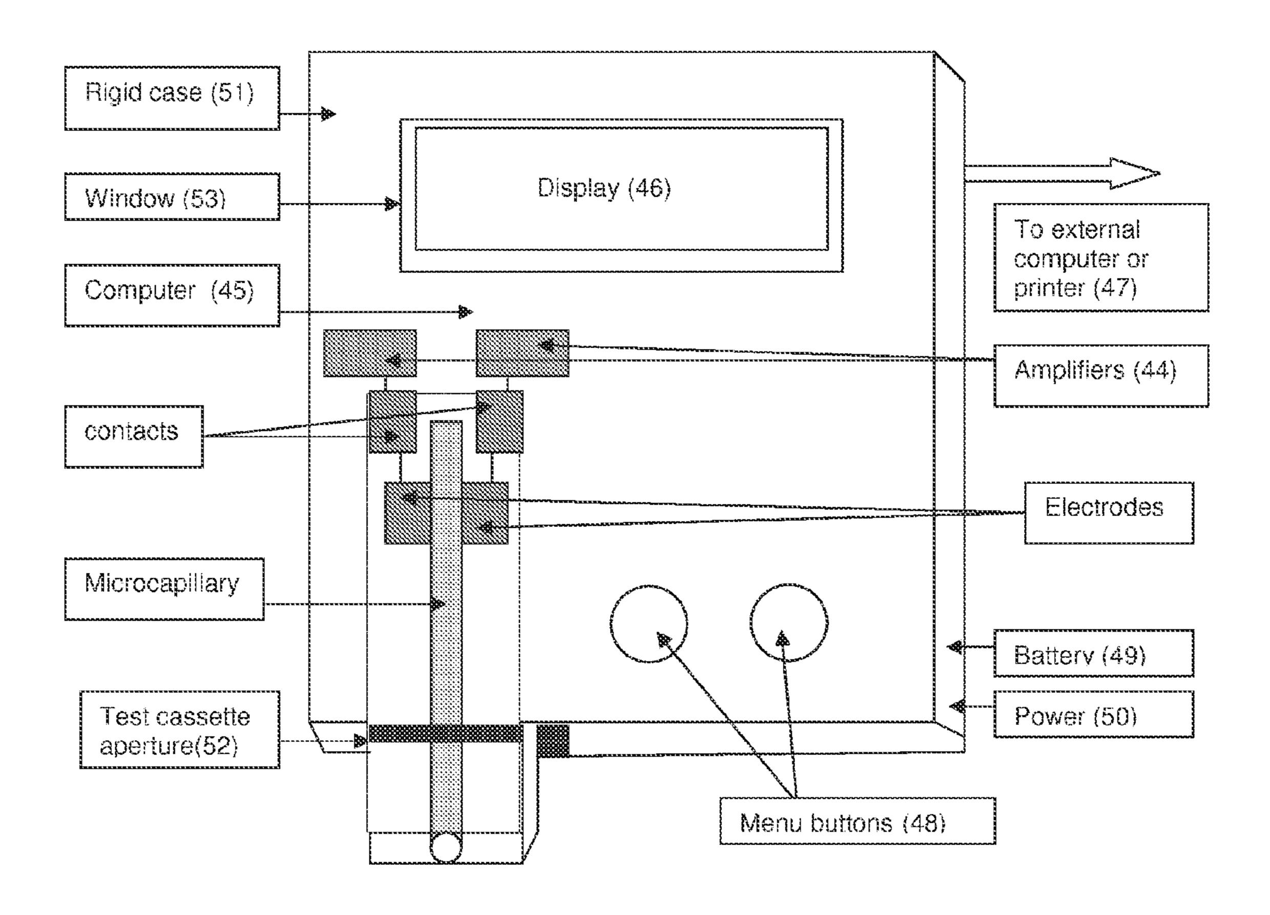
Figure 4b. Biosensor Instrument (39)
