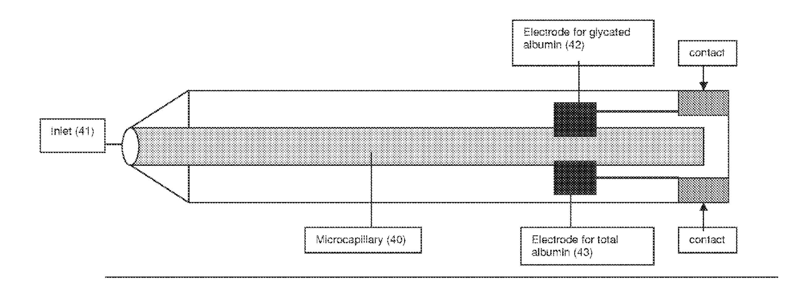
Figure 4 a. Biosensor cassette (38) enlarged.
