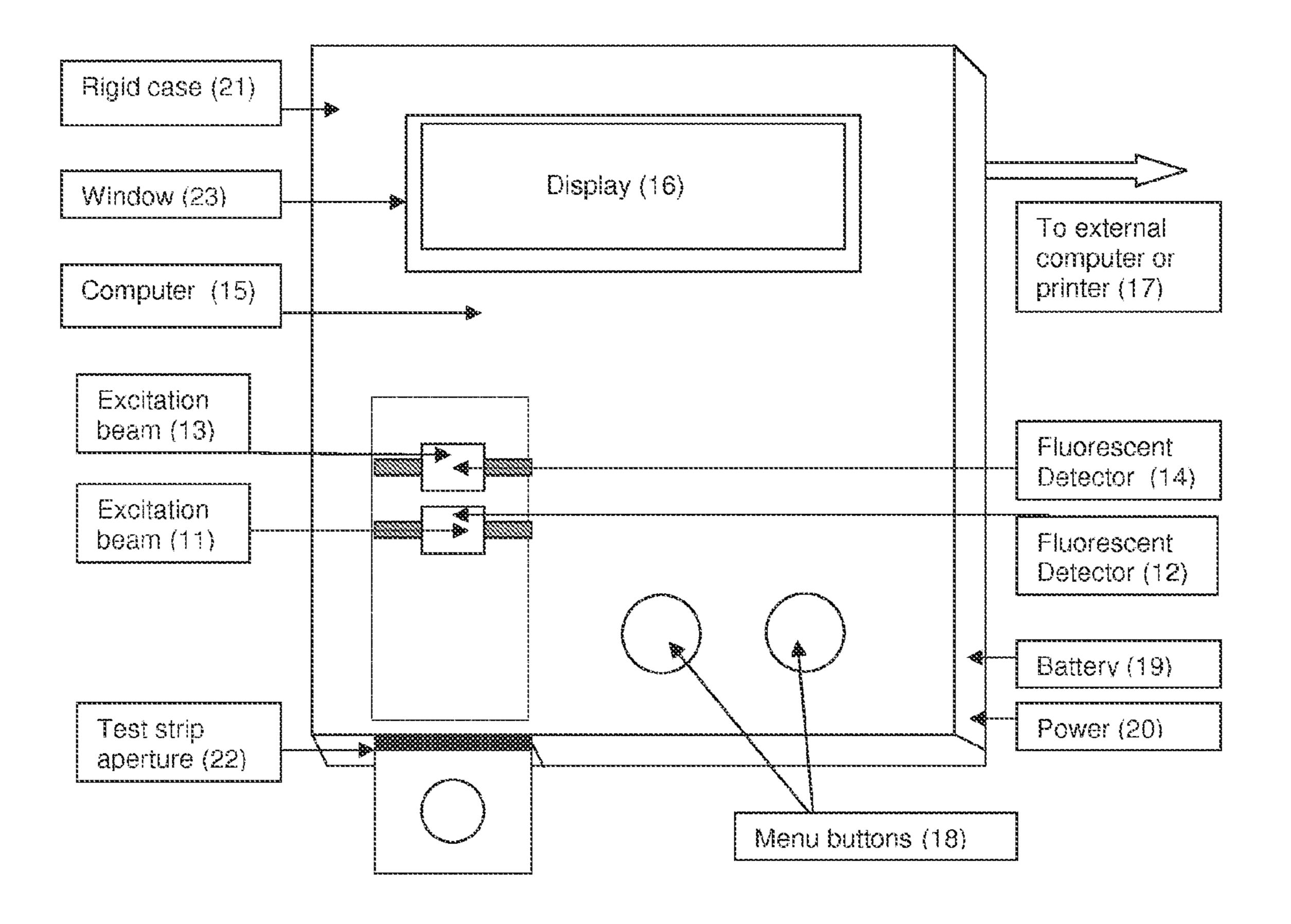
Figure 2. Fluorometer Instrument (10)
