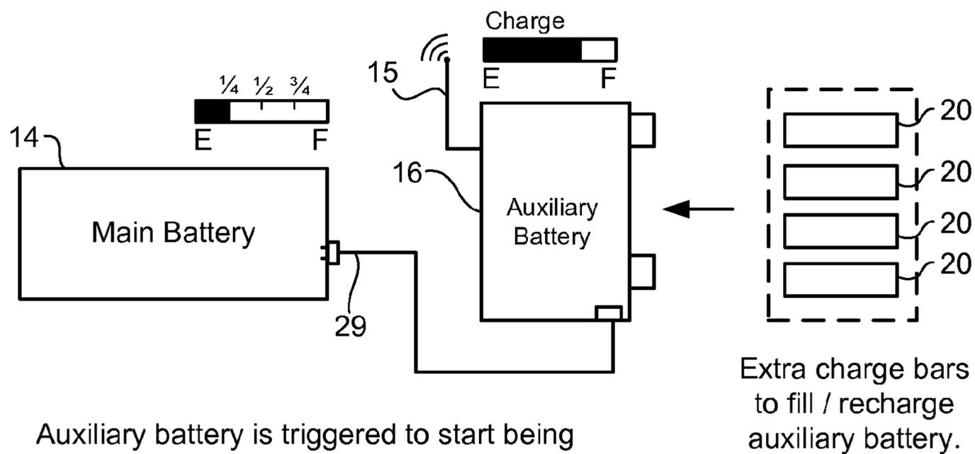
Auxiliary battery is triggered to start being accessed for power after main battery reaches an empty threshold (e.g. 1/4 charge or less).
