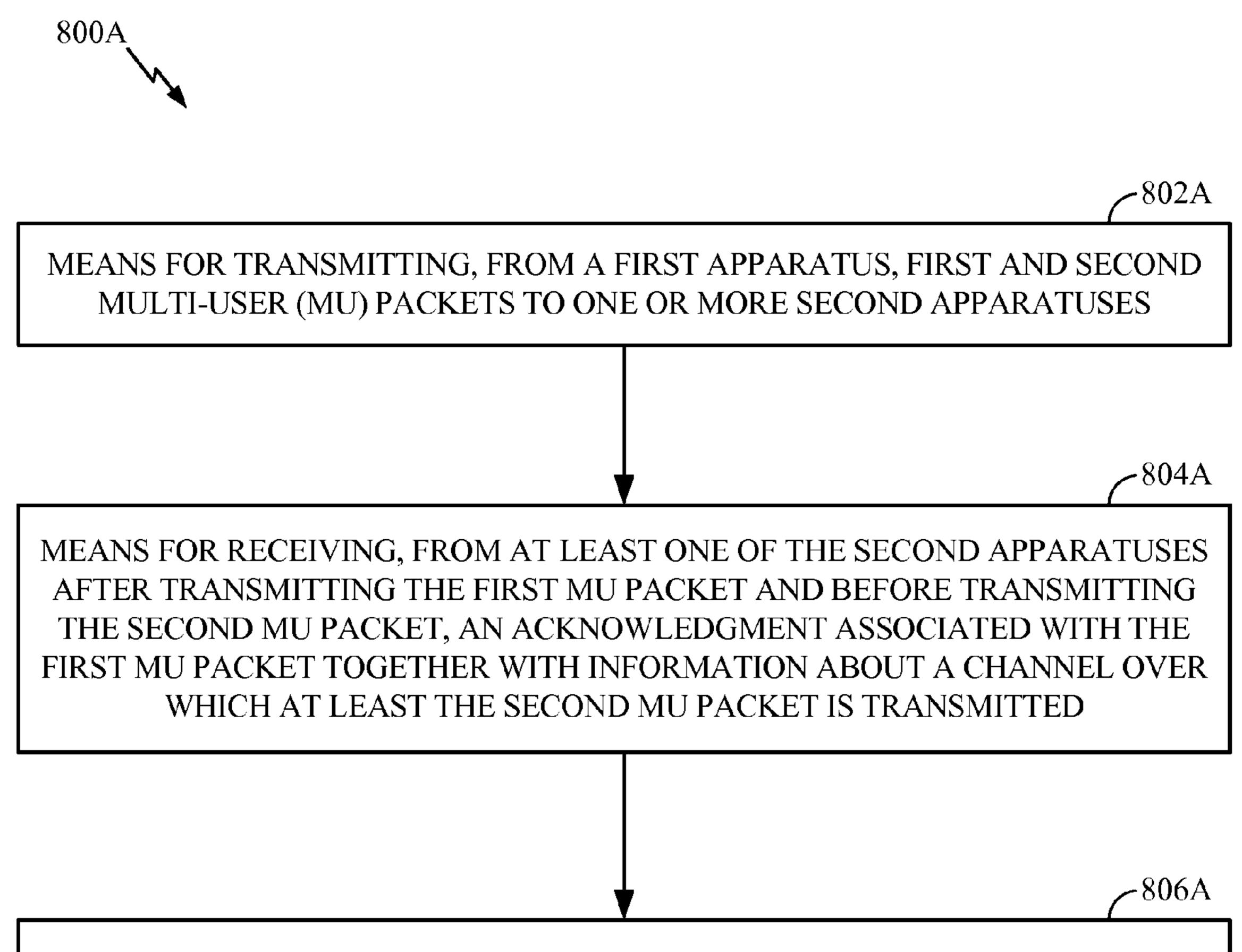
MEANS FOR TRANSMITTING, TO THE AT LEAST ONE OF THE SECOND APPARATUSES, AN ACKNOWLEDGEMENT REQUEST AND AT LEAST ONE OF A NULL DATA PACKET ANNOUNCEMENT (NDPA) OR A SOUNDING POLL, WHEREIN THE MEANS FOR RECEIVING IS CONFIGURED TO RECEIVE, FROM THE AT LEAST ONE OF THE SECOND APPARATUSES IN RESPONSE TO TRANSMITTING THE ACKNOWLEDGMENT REQUEST, THE ACKNOWLEDGMENT TOGETHER WITH THE INFORMATION ABOUT THE CHANNEL
