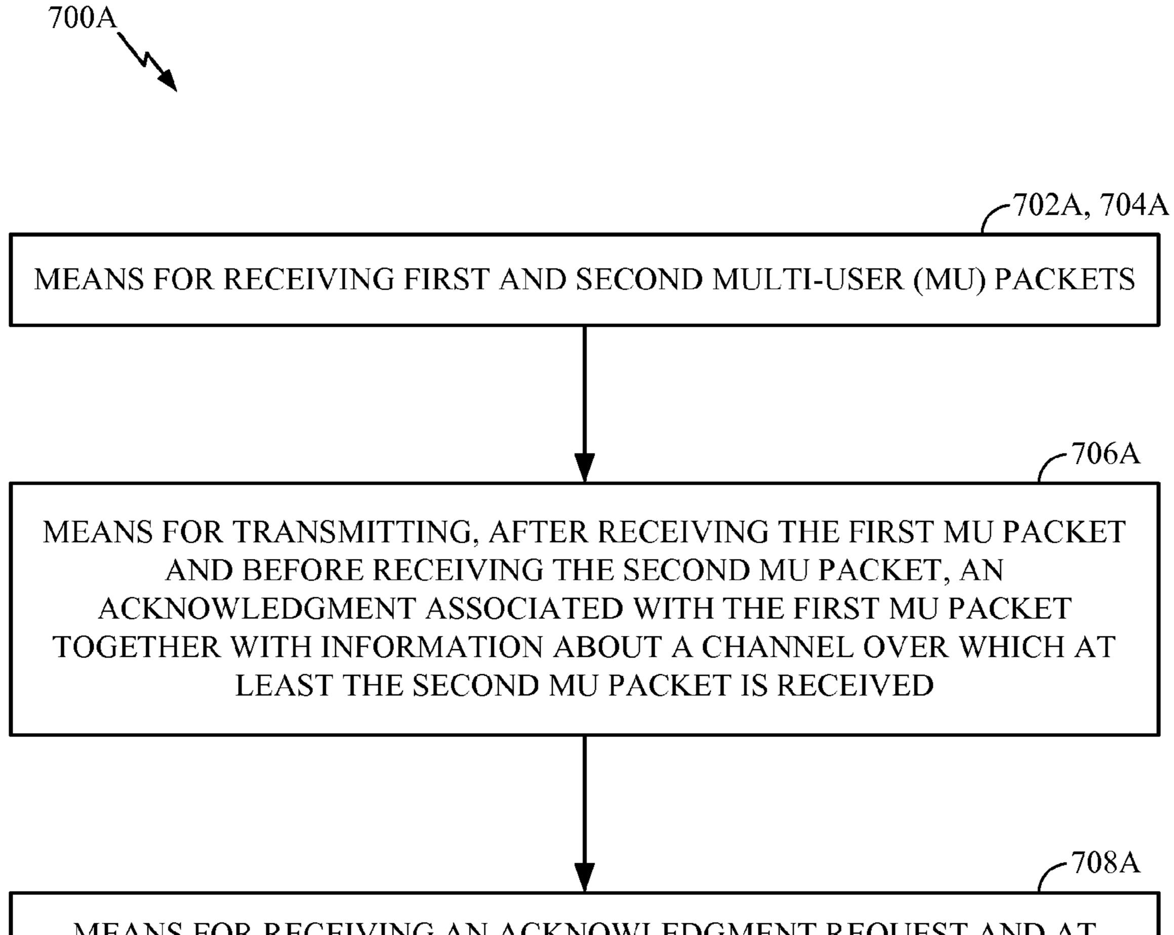
MEANS FOR RECEIVING AN ACKNOWLEDGMENT REQUEST AND AT LEAST ONE OF A NULL DATA PACKET ANNOUNCEMENT (NDPA) OR A SOUNDING POLL, WHEREIN THE MEANS FOR TRANSMITTING IS CONFIGURED TO TRANSMIT THE ACKNOWLEDGMENT TOGETHER WITH THE INFORMATION ABOUT THE CHANNEL IN RESPONSE TO RECEIVING THE ACKNOWLEDGMENT REQUEST
