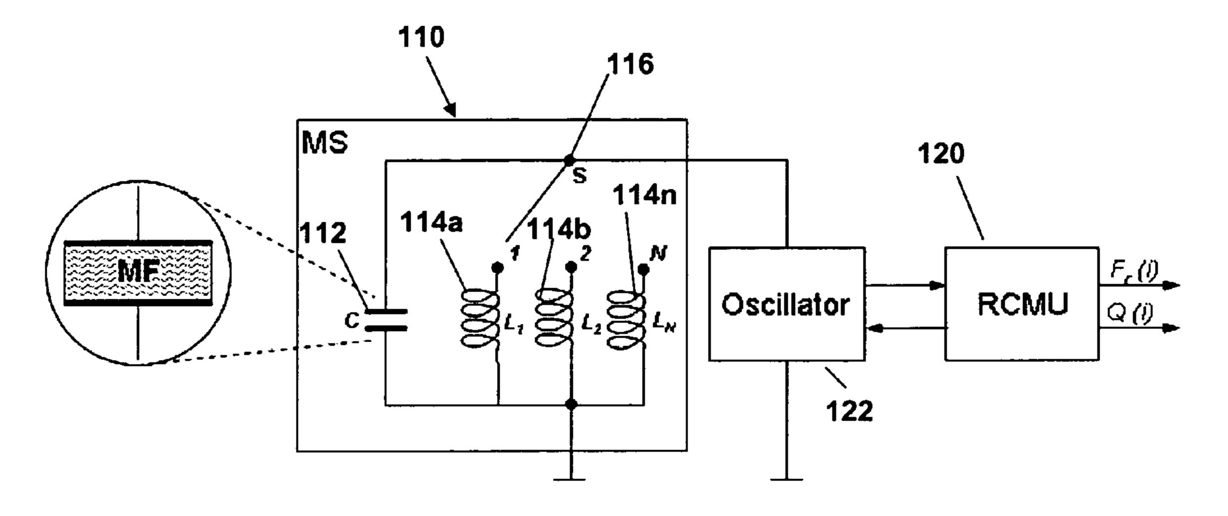
MS - measuring sensor (LCR Measuring Circuit)
