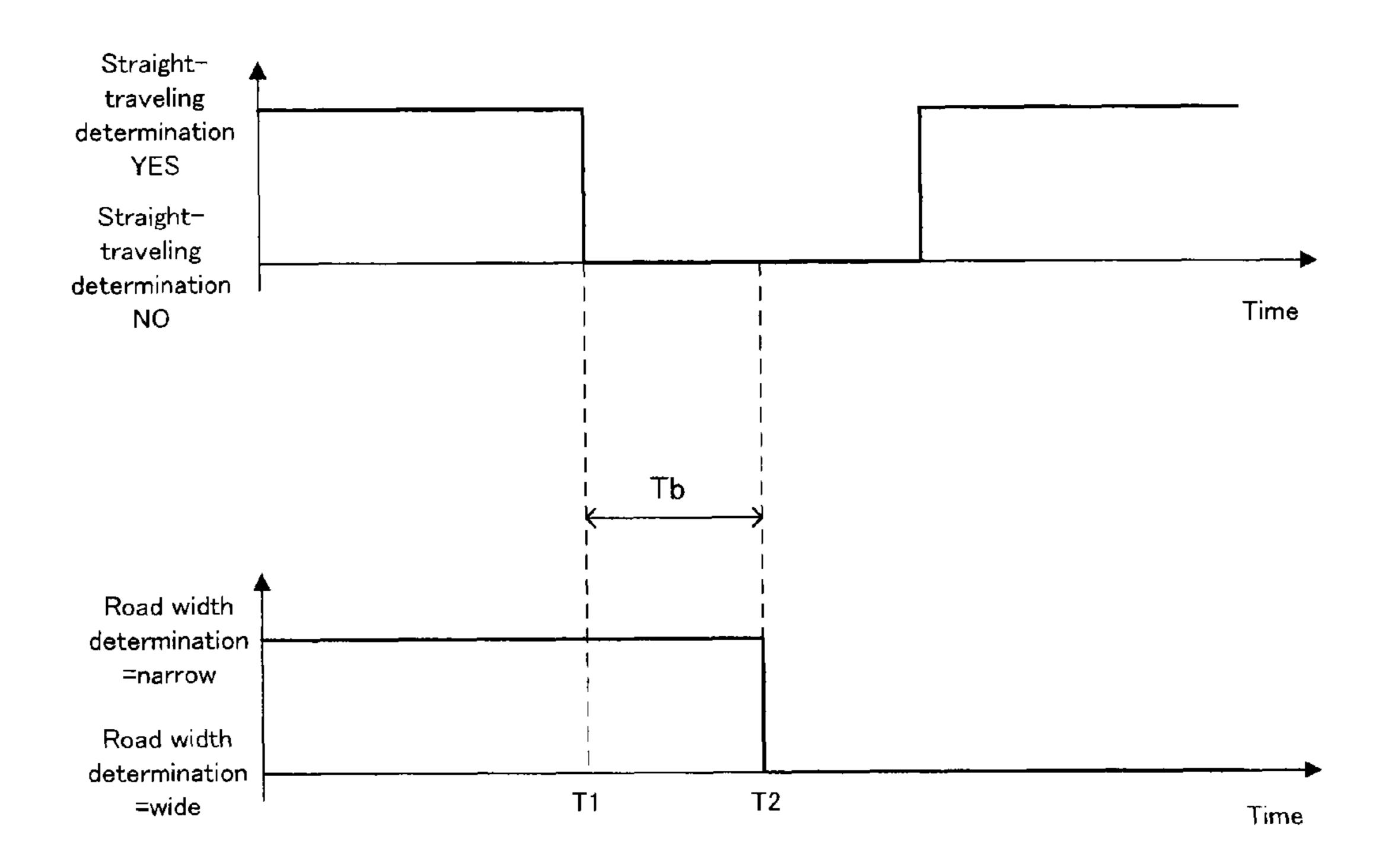
Road width determination=narrow (small steering reaction force)
