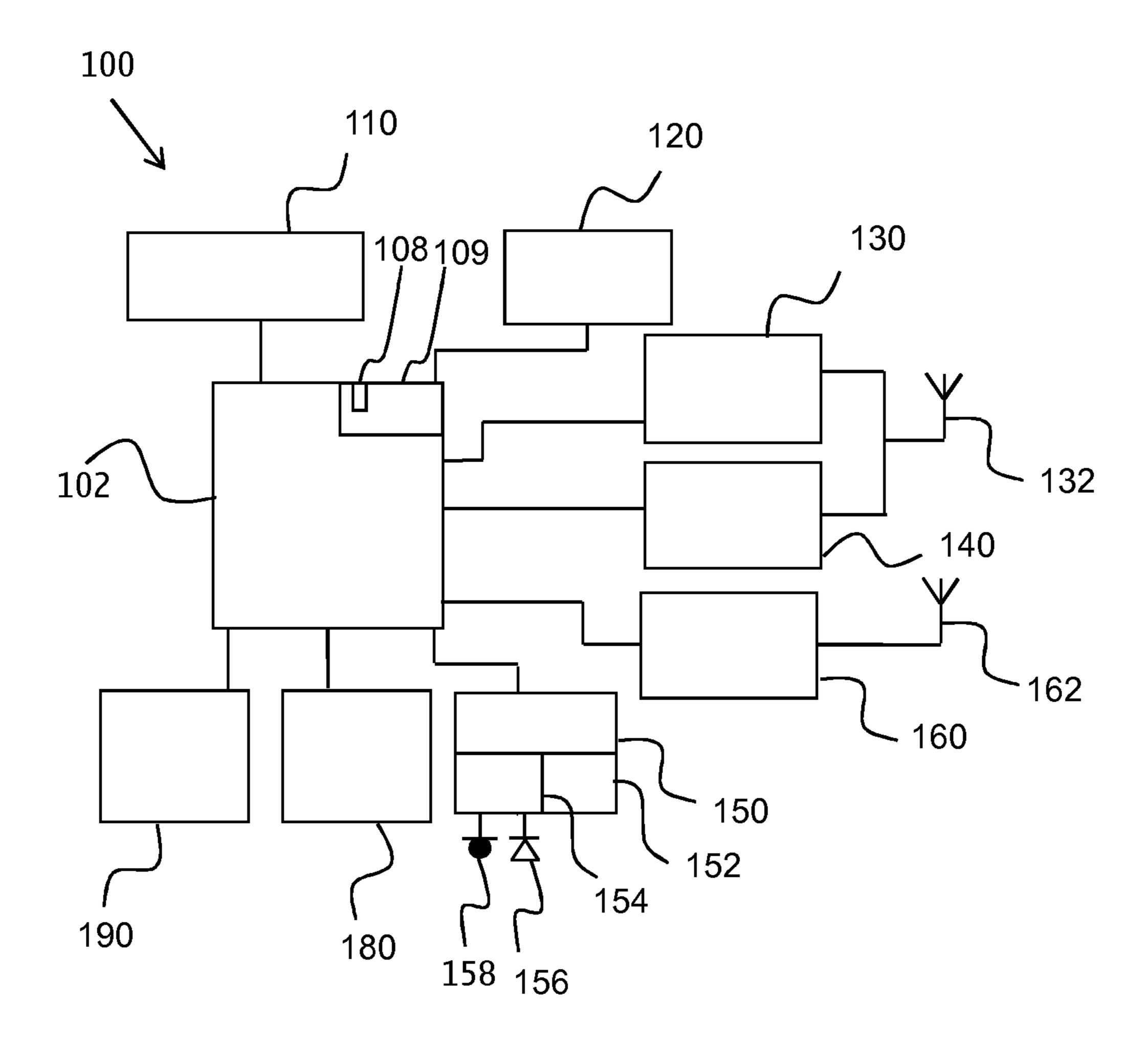
100 – Host / Mobile phone 160 – FM transmitter 102 – Control unit 162 – FM transmitter antenna 110 – Memory 180 – **Display** 120 – Battery 190 – Input devices (keyboard/touchpad) 150 – Audio circuitry 109 – Energy Mgt. Circuit 108 – Charging connector 154 – Audio in/out internal 158 – Microphone 130 – Cellular transmitter 140 – Cellular receiver 156 – Loudspeaker 132 – Cellular antenna 152 – Audio in/out external
