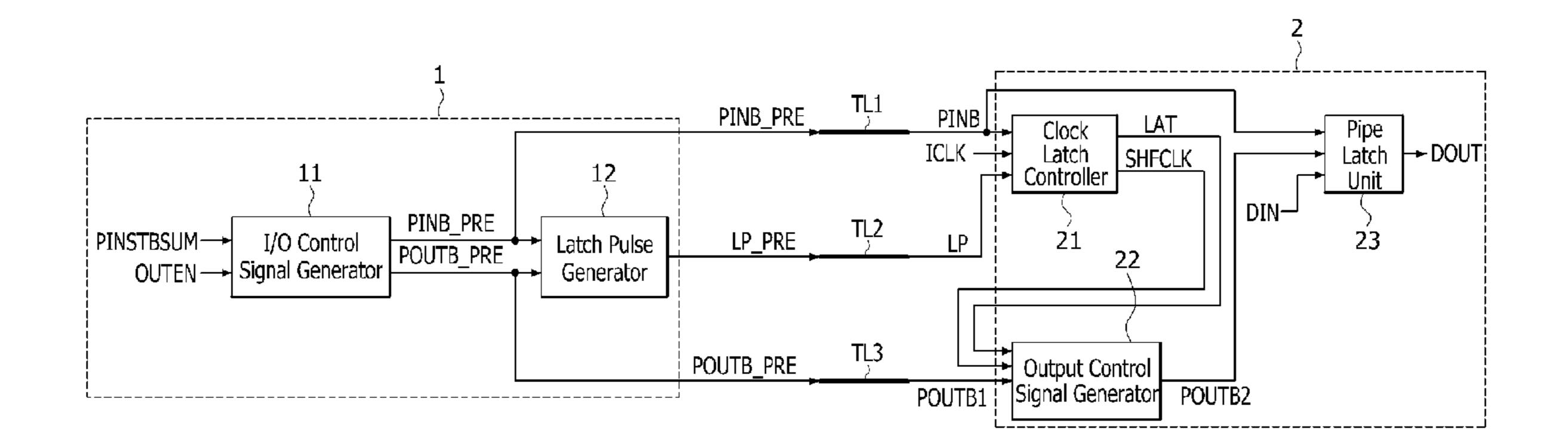
$\sim$ Signal Generator Clock Latch Controller PINB <u>ك</u> മ Latch Pulse Generator I/O Control Signal Generator TBSUM-OUTEN-
