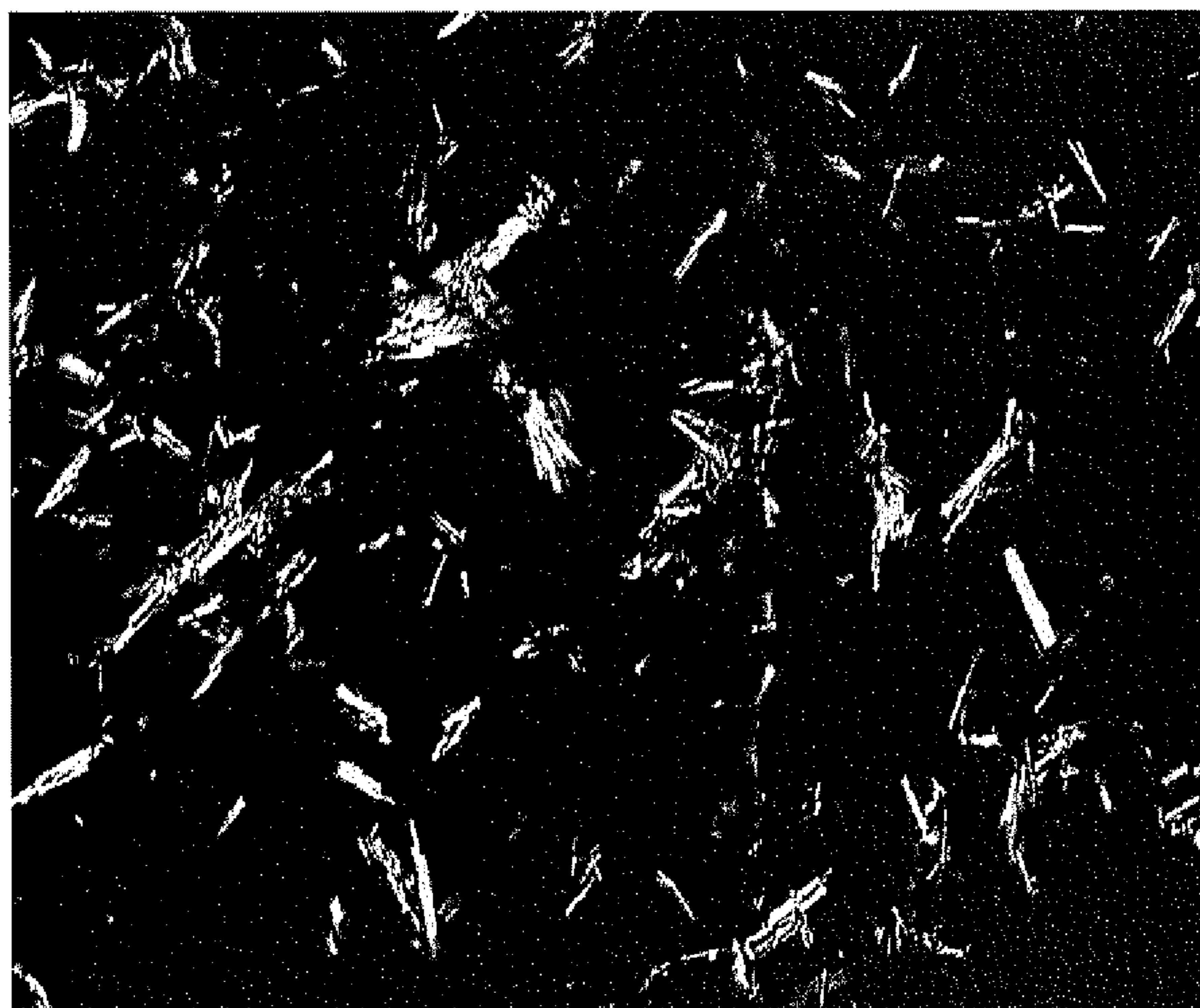
Crossed Polarized: Birefringence Observed
