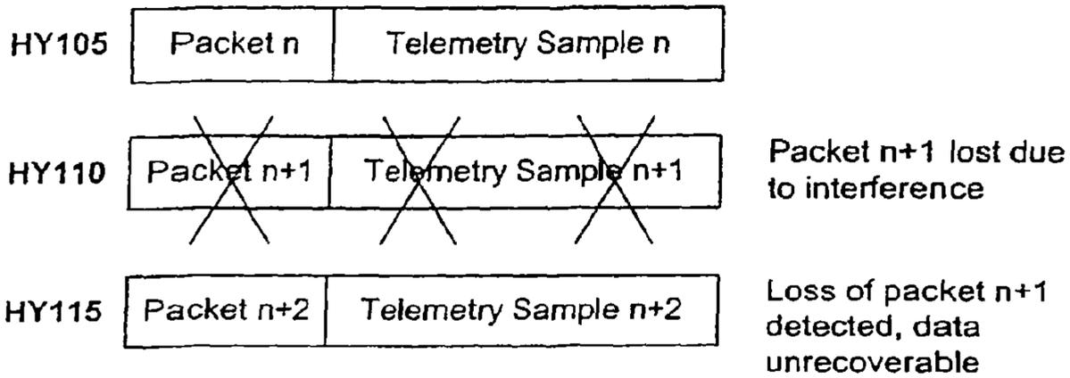
Probability of Telemetry Sample Loss ( $P_{TSL}$ )
