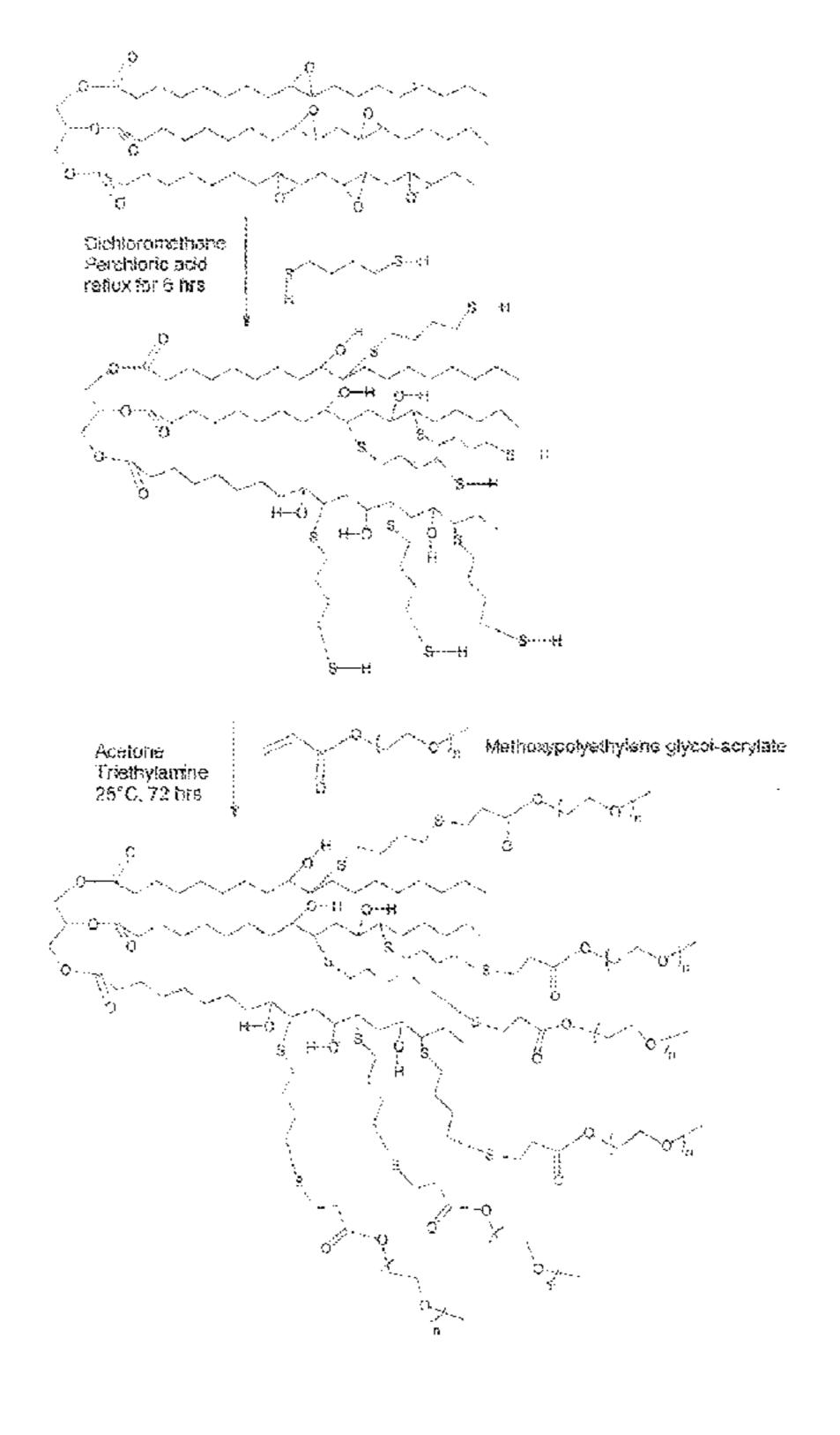
Schematic representation of preparation of surfactant derived from epoxidized
