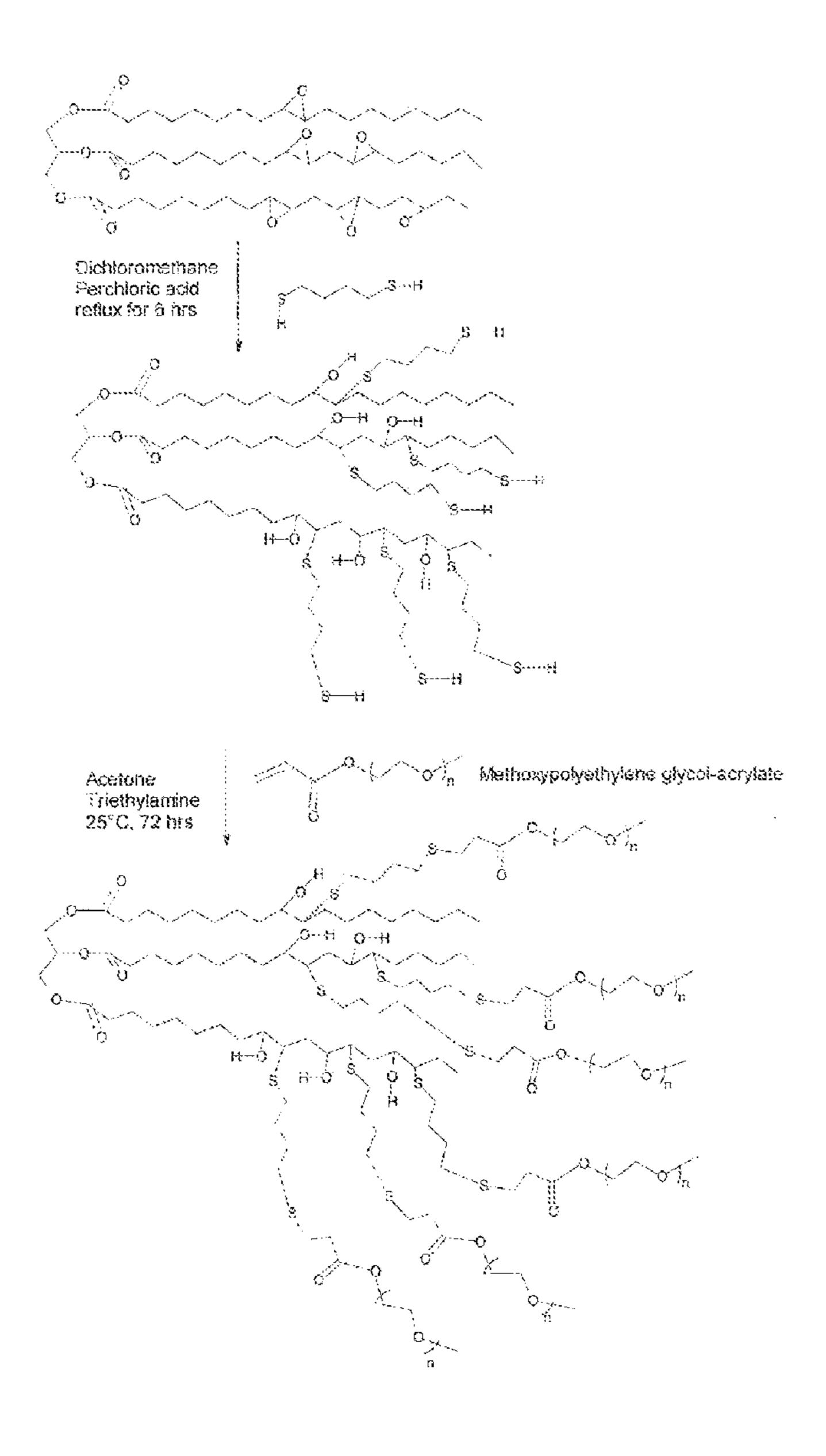
Figure 1: Schematic representation of preparation of surfactant derived from epoxidized soybean oil, thioether bond forming linker, and water soluble polymer.
