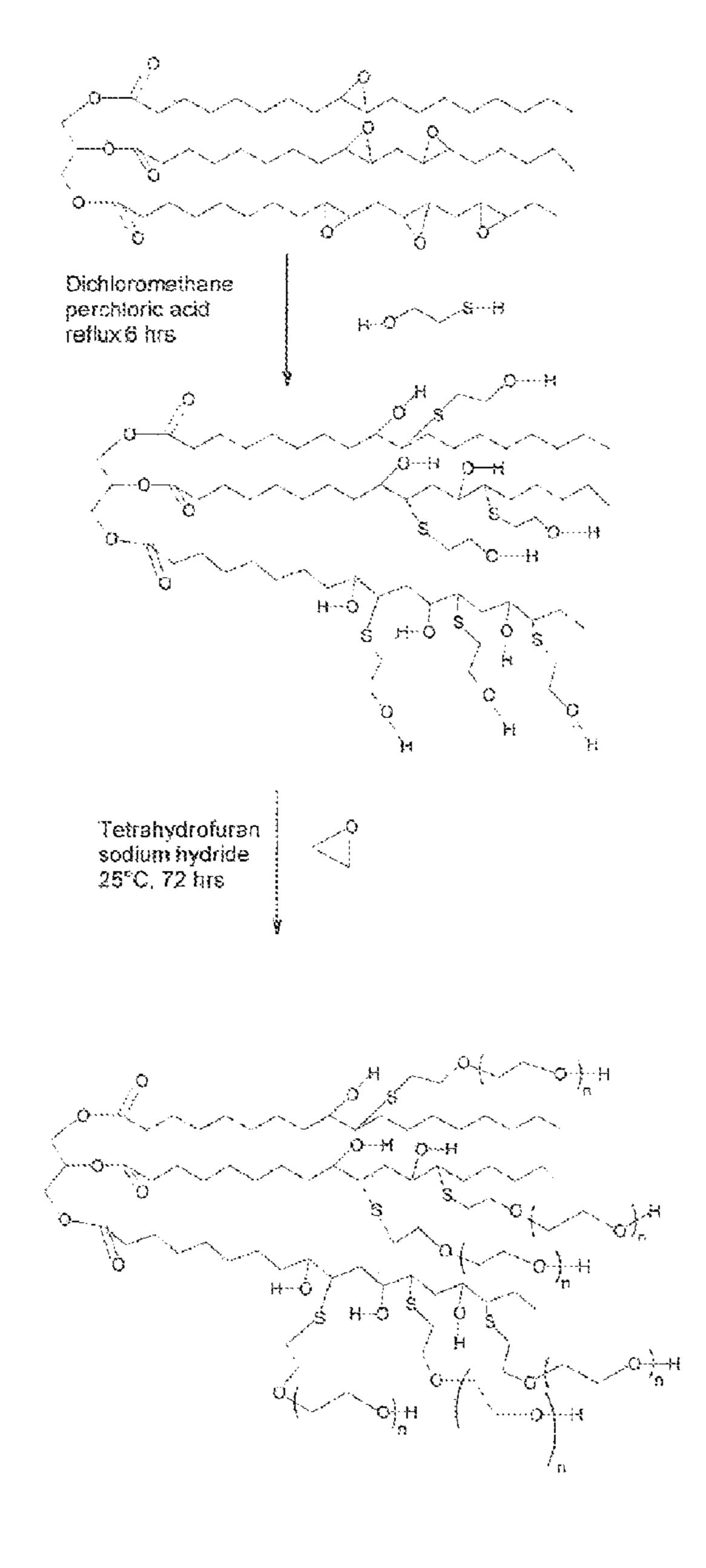
Figure 3: Schematic representation of preparation of surfactant derived from epoxidized soybean oil, thioether bond forming linker and monomer polymerization initiated by linker.
