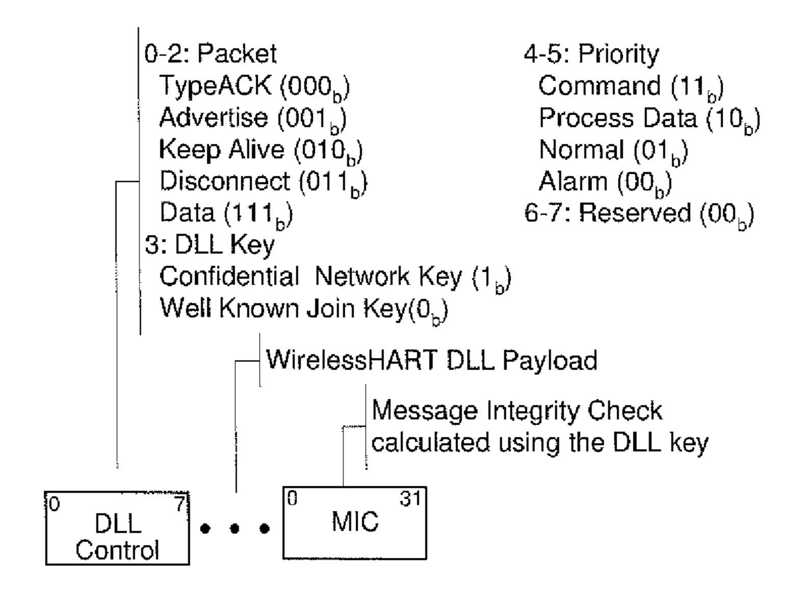
FIG. 5 Wireless HART DLL Header
