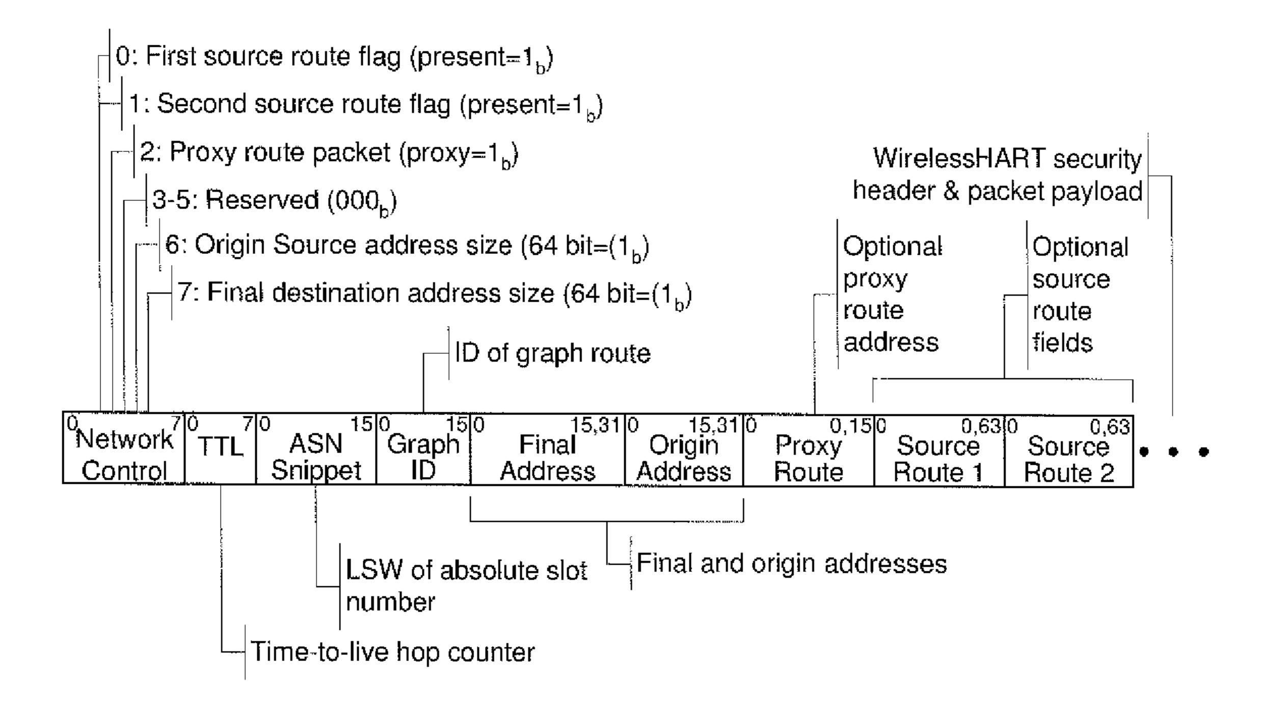
FIG. 7 WirelessHART Network Header
