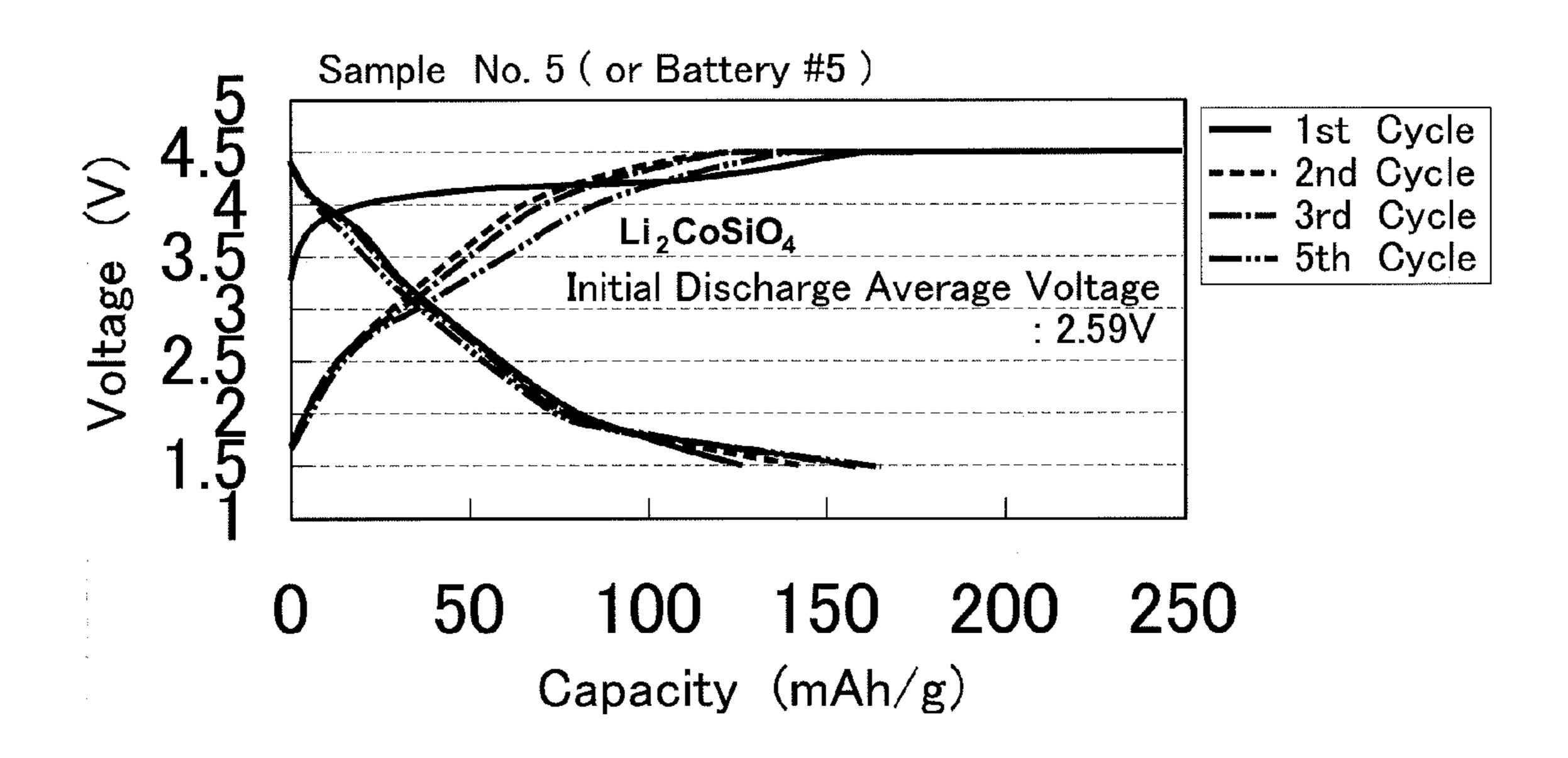
LITHIUM SILICATE-BASED COMPOUND AND PRODUCTION PROCESS FOR THE SAME, POSITIVE-ELECTRODE ACTIVE MATERIAL AND POSITIVE ELECTRODE FOR USE IN LITHIUM-ION SECONDARY BATTERY AS WELL AS SECONDARY **BATTERY**
