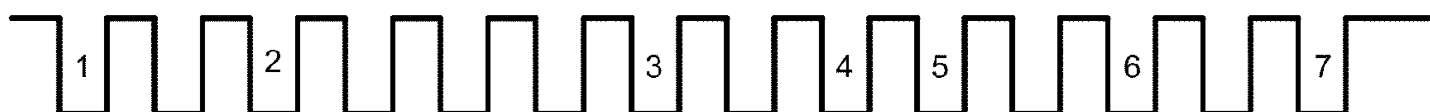
INTERRUPT TIMING WAVEFORM 2 (assuming frequent servicing events w/o aperture)
