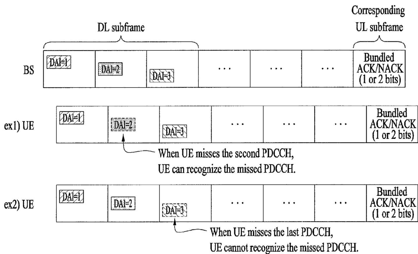
\* When ACK/NACK is transmitted on PUSCH, UE can recognize whether PDCCH is missed by comparing DAI (DL-DAI) with DAI (UL-DAI) of UL grant PDCCH.
