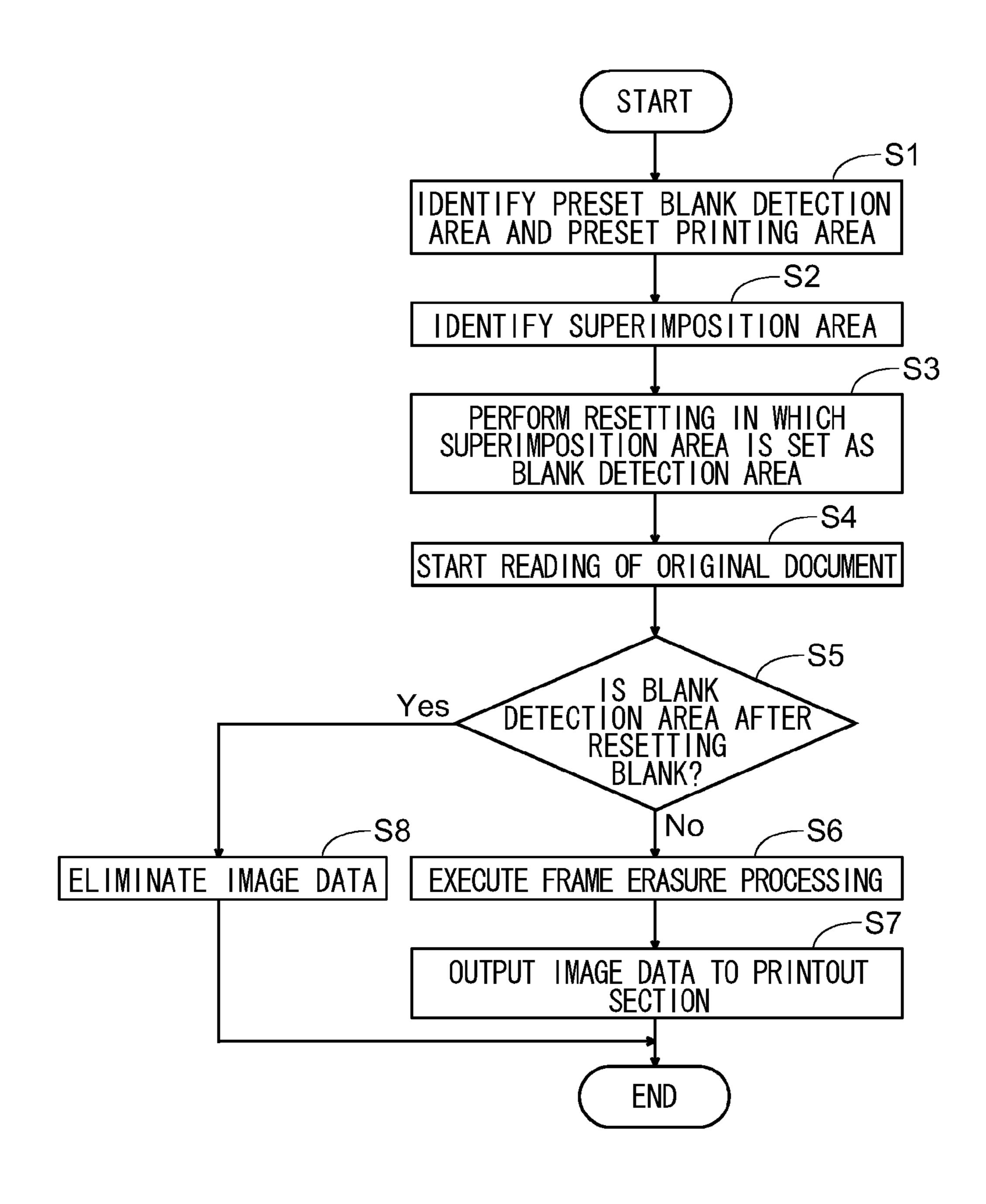
IMAGE READING DEVICE CAPABLE OF EXECUTING BLANK ELIMINATION PROCESSING AND FRAME ERASURE PROCESSING AND AN IMAGE FORMING APPARATUS INCLUDING THE SAME
