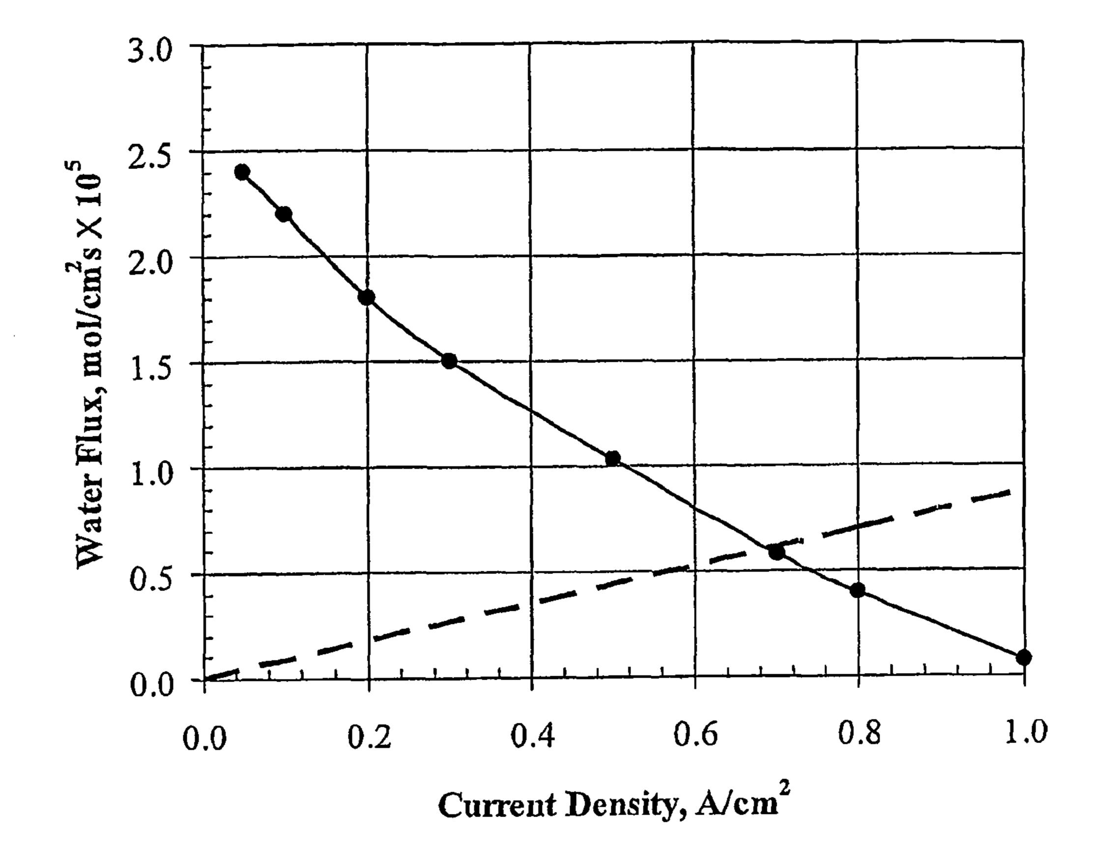
Figure 5: Flux of water across a 115 Nafion membrane as a function of current density (T = 80°C). The symbols are the data obtained experimentally for the HCl electrolyzer. The dashed line is the stoichiometric amount of water required in Reaction [1] (oxidation of SO<sub>2</sub> to H<sub>2</sub>SO<sub>4</sub>).
