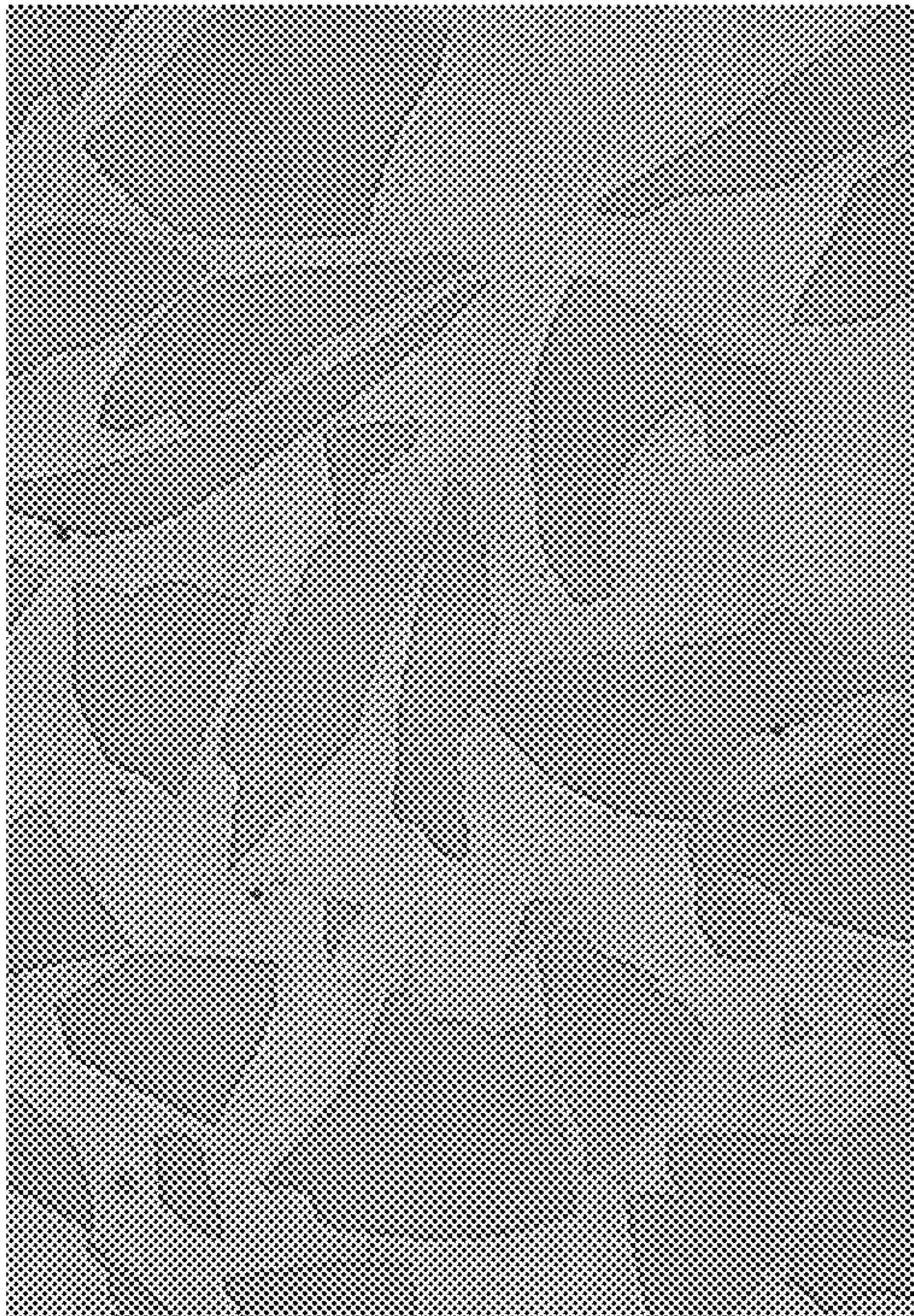
FIG. 2A - Binderless WC infiltrated with Cu alloy
