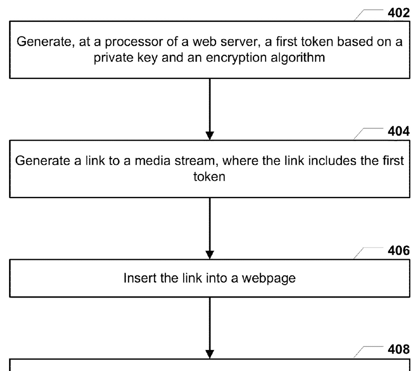
Send the webpage from the web server to a client device, where selection of the link causes a media request to be sent to a media server associated with the media stream, where the media request includes the first token, and where the media request is granted or denied based at least in part on whether a second token generated in response to the media request matches the first token
