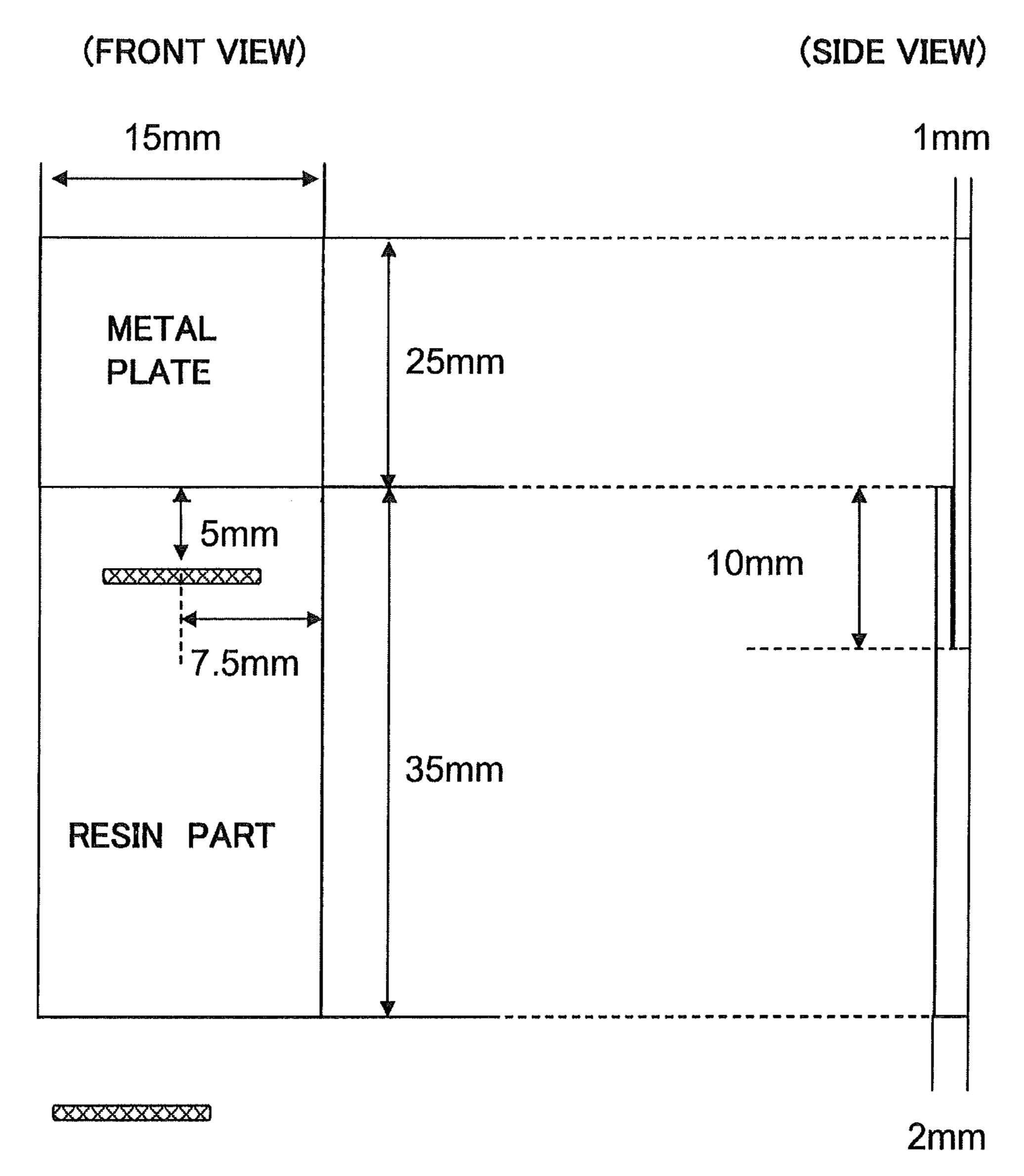
PORTION WHERE JIG FOR BENDING TEST WAS APPLIED
