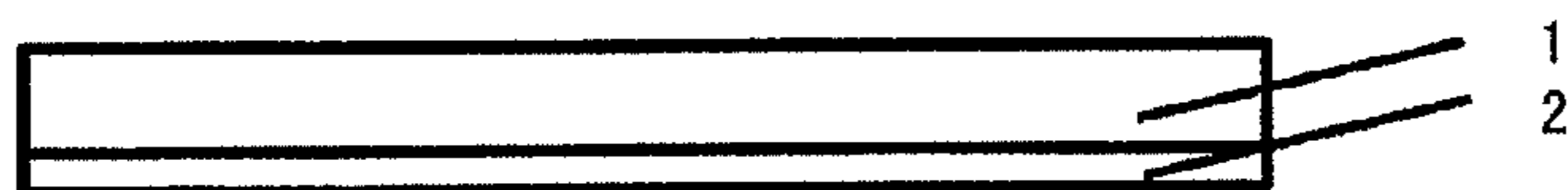
Fig.1 cross-section drawing of biaxially oriented film and adherent layer
