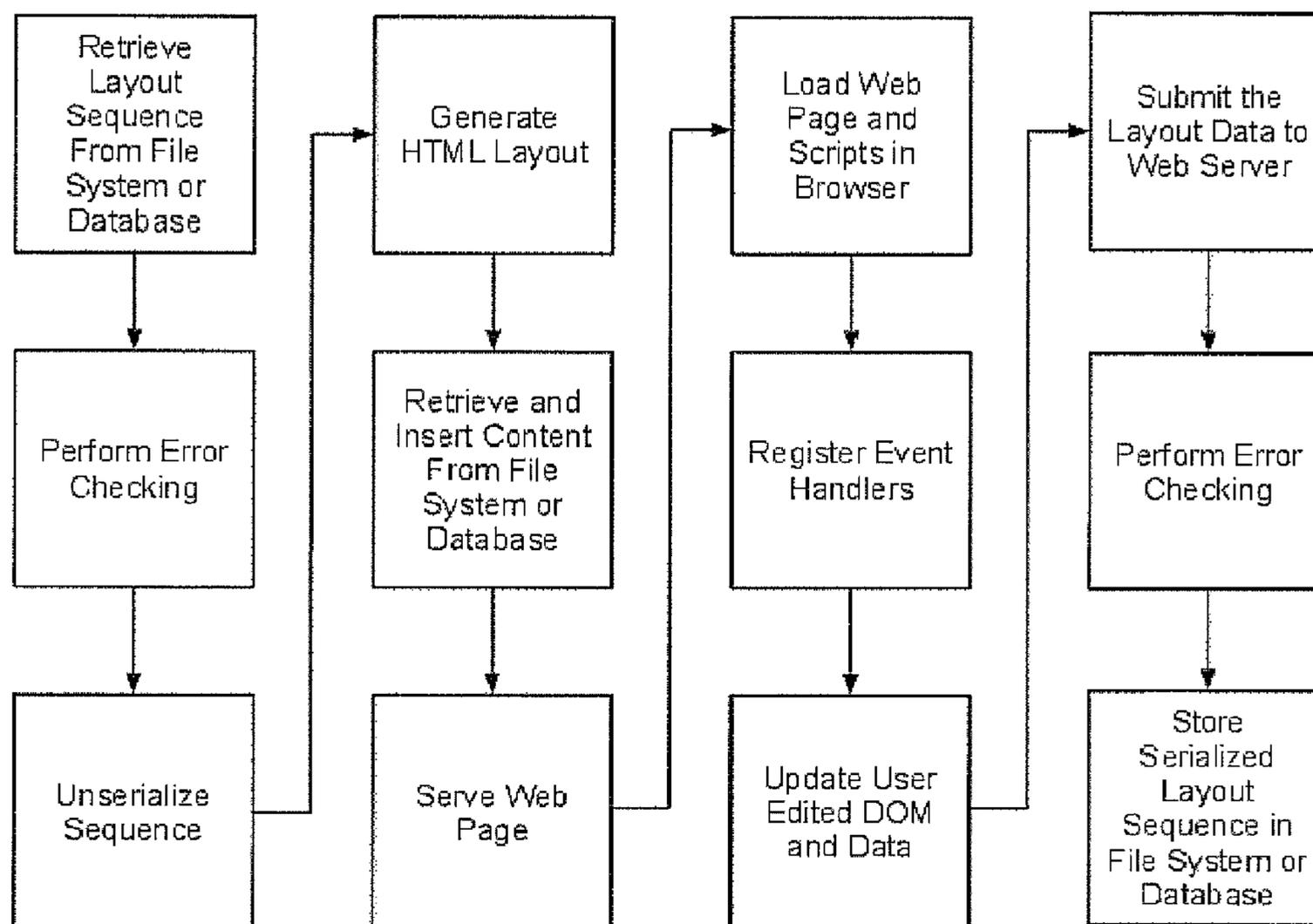
Figure 22 - Application Logic Sequence
