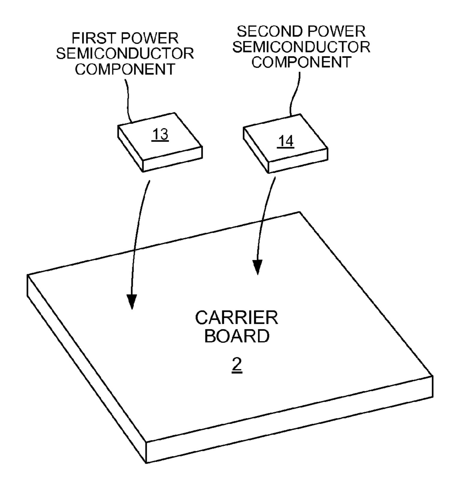
MOUNTING FIRST AND SECOND POWER SEMICONDUCTOR COMPONENTS ONTO CARRIER BOARD
