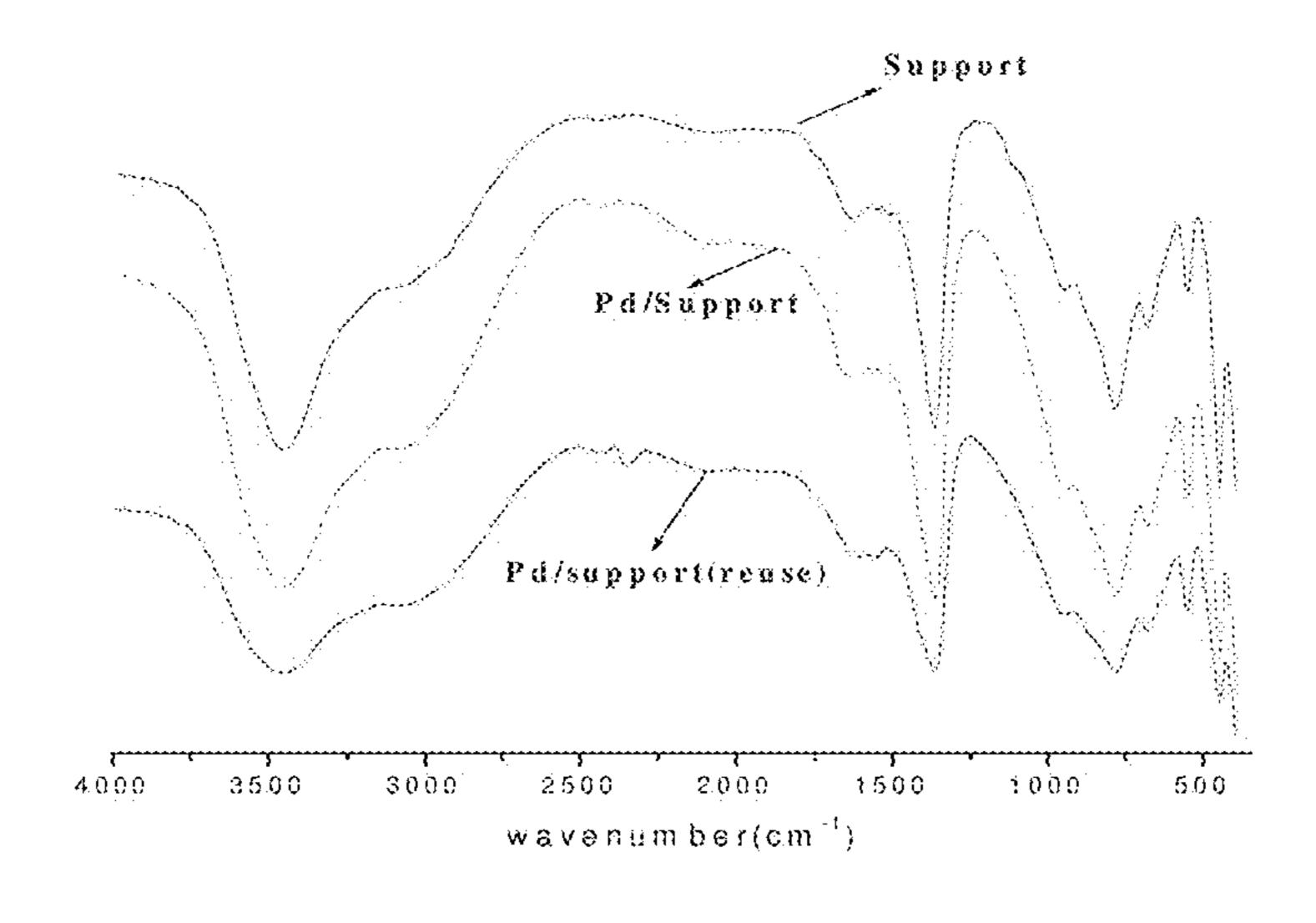
Fig. 2 FTIR spectra of the support and catalysts.
