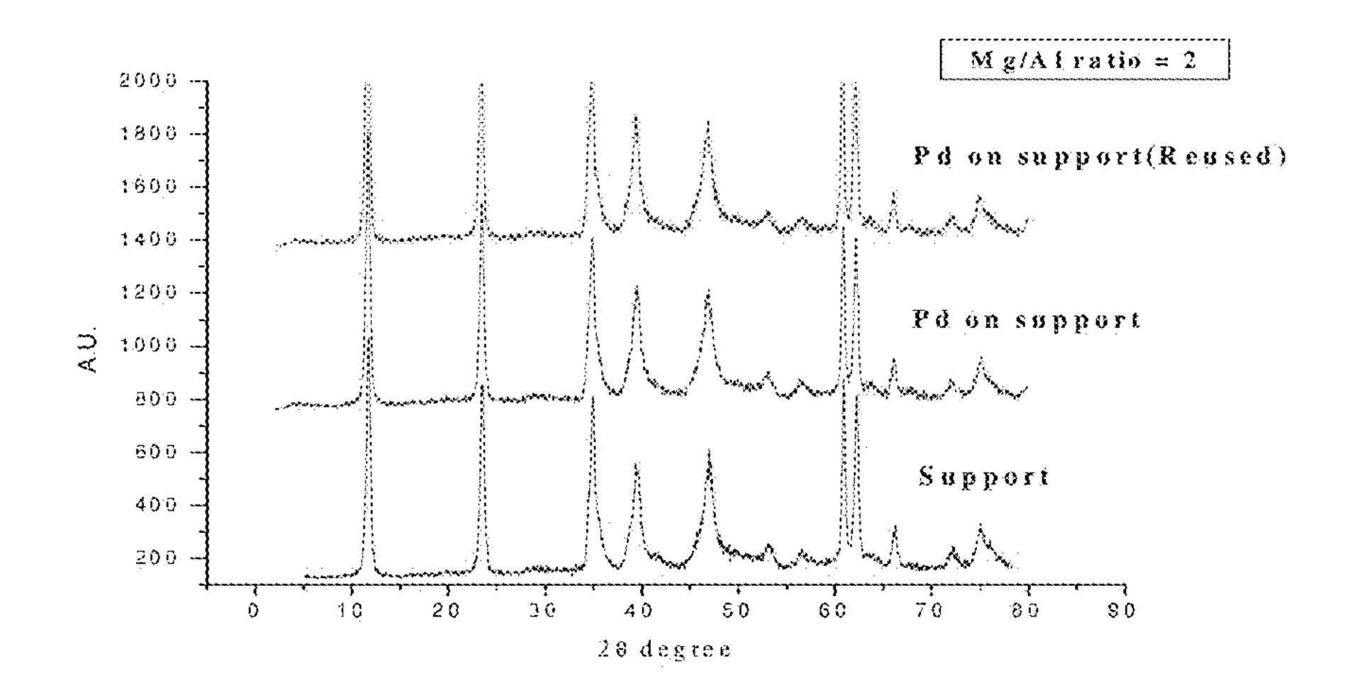
Fig. 1 XRD patterns for the support and catalyst
