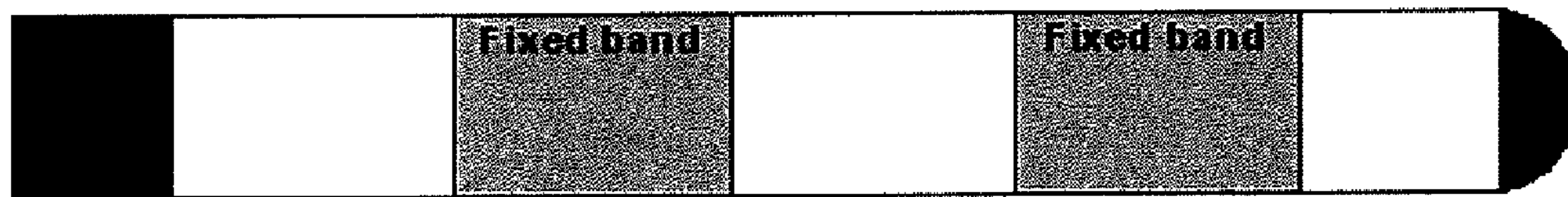
Prior art cigarette wrapper with fixed banded regions (FB) of reduced permeability
