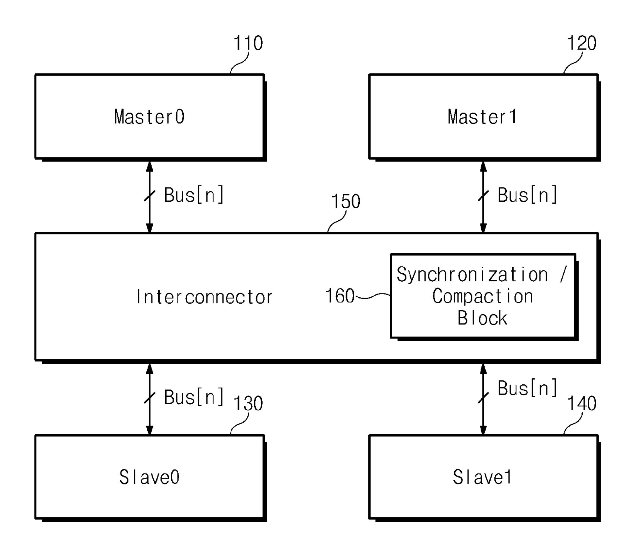
Slave0 Payload Channe Data Channel / Channel) } Ready Channel) d Request Cha (AR Channel) Data Char 3 Channel Response (B Channe Write Request (AW Chann Read  $\geq$ 150 d Request Channel (AR Channel) Data Channel / Channel) Ready channe | |-Response (B Channe Write Request (AW Chann Read
