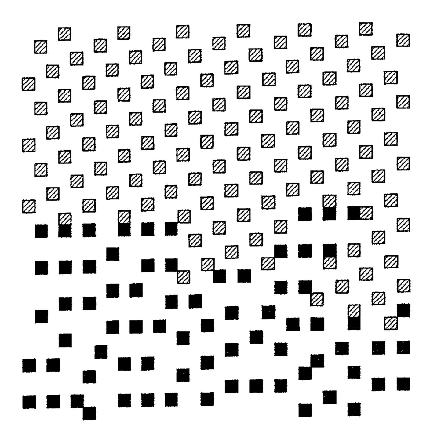
□ : DOT PIXEL OF ERROR-DIFFUSED IMAGE□ : DOT PIXEL OF SCREEN-PROCESSED IMAGE
