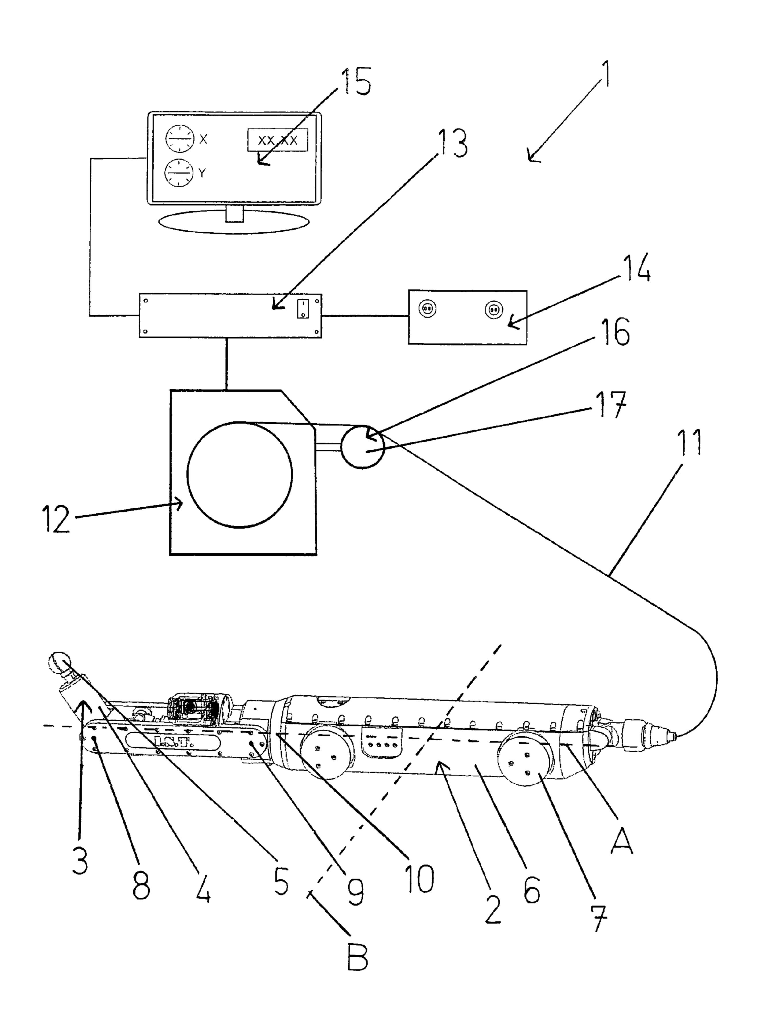
The invention relates to a device for renovating a pipe, the latter being provided with at least one opening arranged in the wall of the pipe, said device having a base unit that can be introduced into the pipe, a clearing unit that is movable relative to the base unit, and an electronic sensor arrangement for
