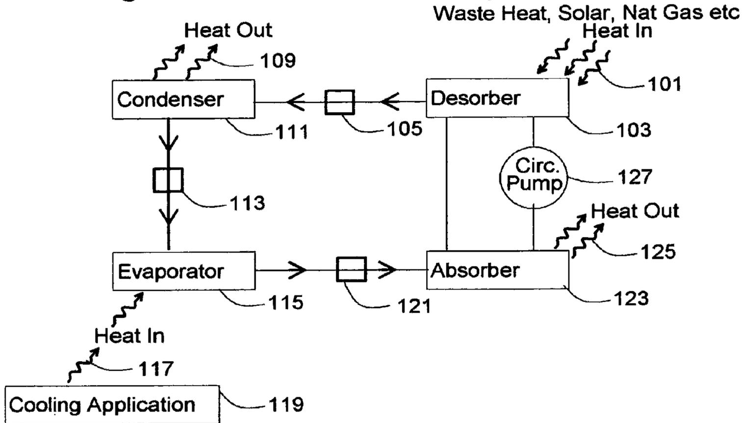
Figure 7b Prior Art - Adsorption Cycle
