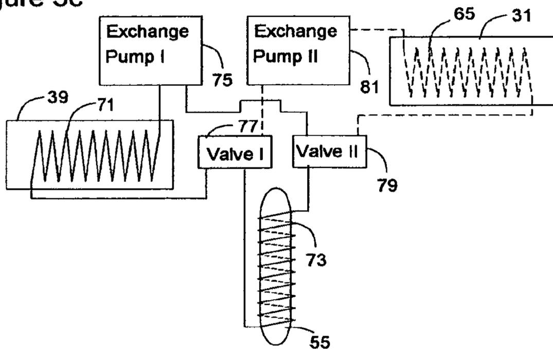
Present Art - Pressure Swing Adsorption Adsorbing and Desorbing
