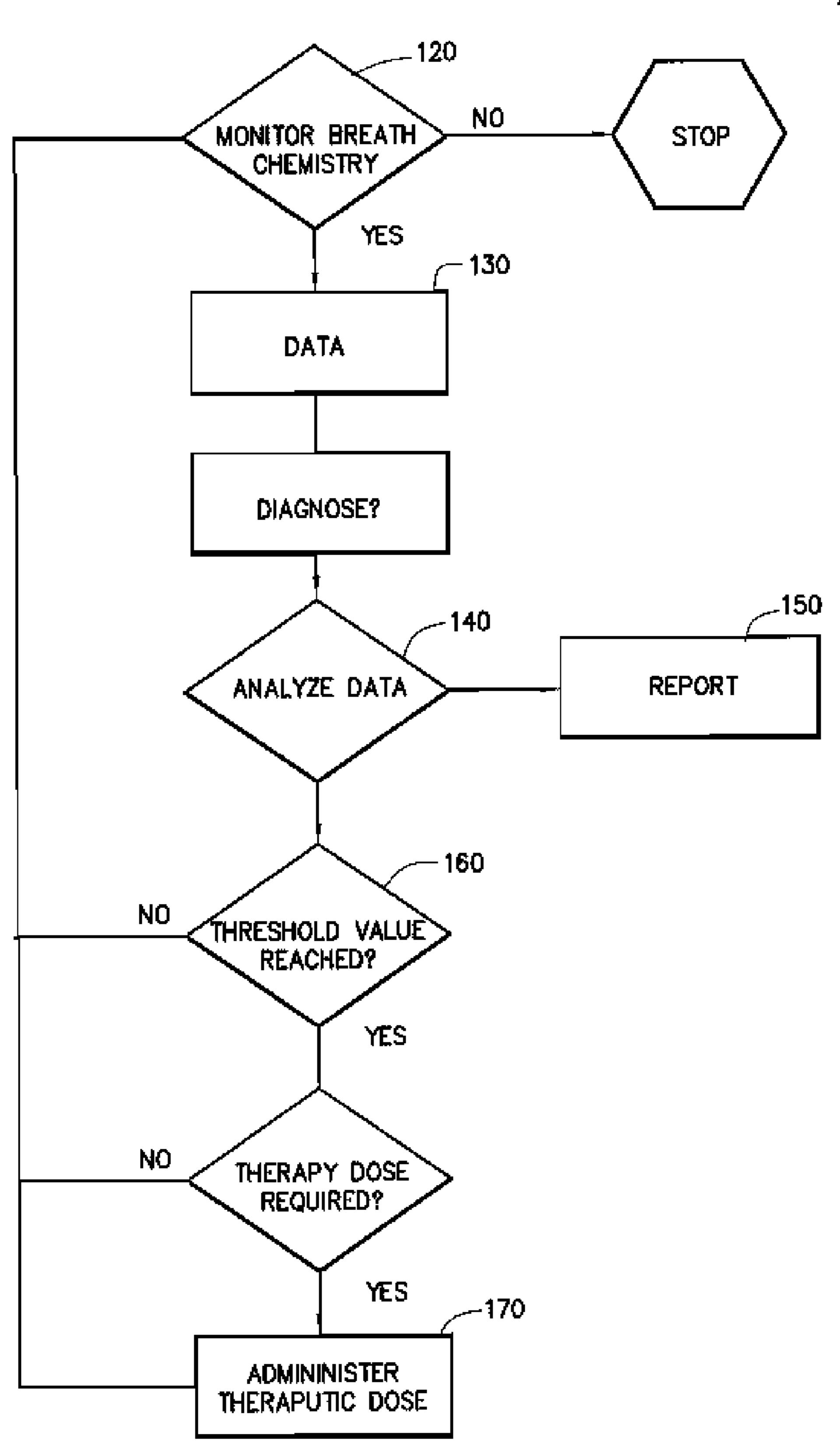
FIG. 13 MONITOR BREATH NO CHEMISTRY AND BREATHING \$TOP YES <del>--</del> 130 DATA DIAGNOSE? 150 140 ANALYZE DATA REPORT 160 NO THRESHOLD VALUE > YES NO THERAPY DOSE REQUIRED? YES ADMINISTER
