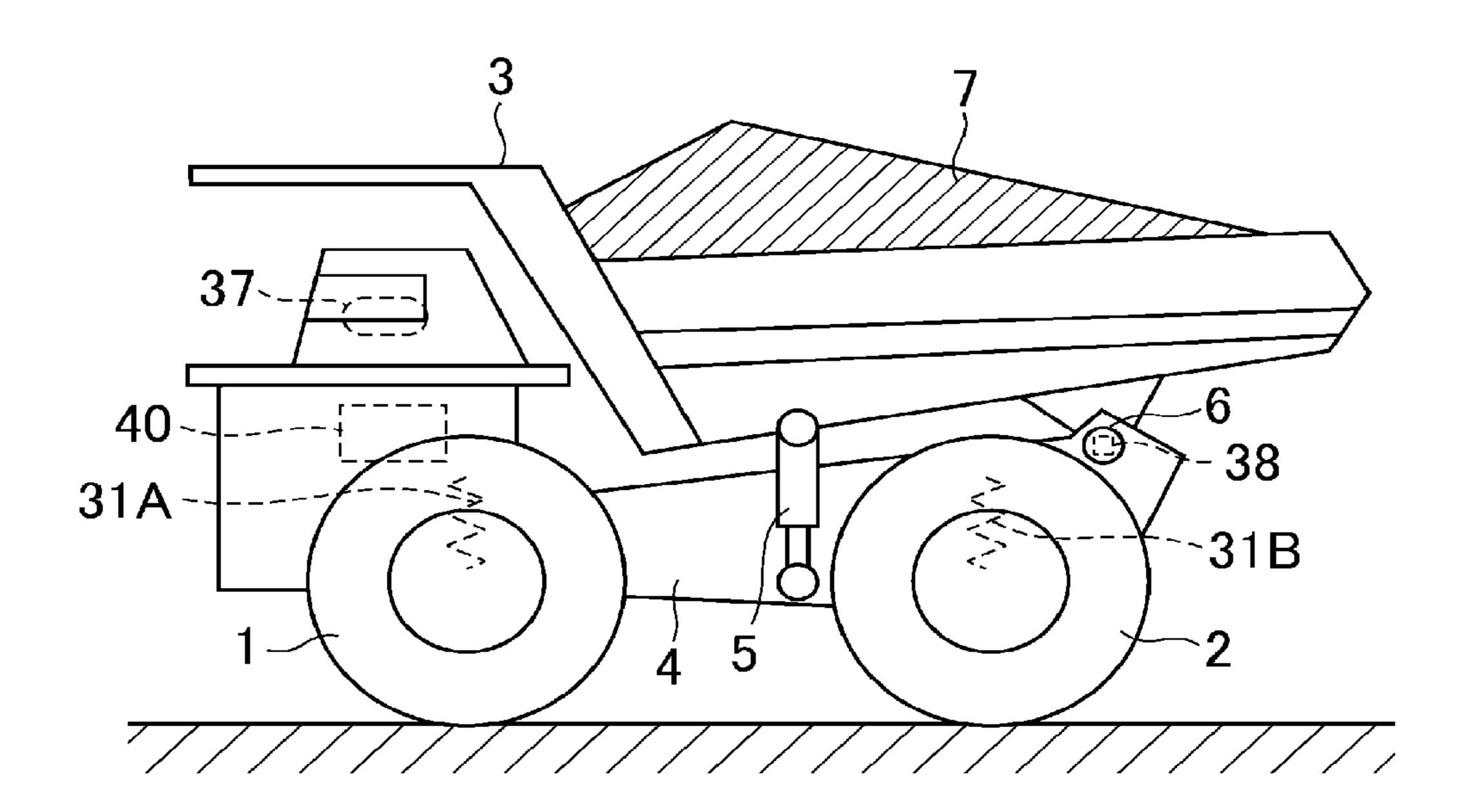
39 36 35 REFERENCE MOMENT CALCULATIO UNIT FRONT AXLE LOAD SENSOR REAR AXLE LOAD SENSOR **POTENTIOMET** 38
