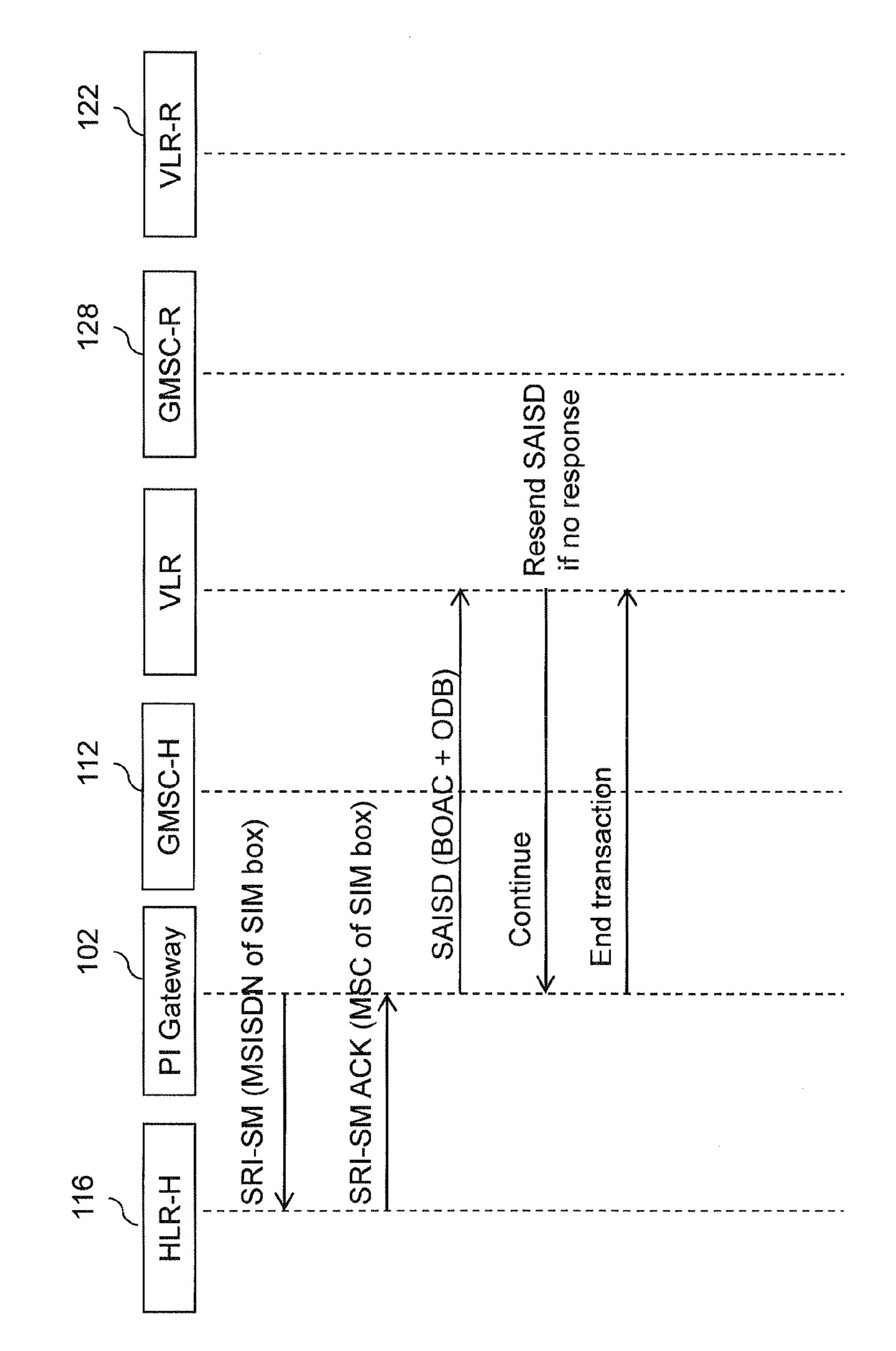
128 Interconnect call blocking for off-net simboxes 102 Pl Gateway 16 offnet Simbox DB If A is not in Simbox DB offnet
