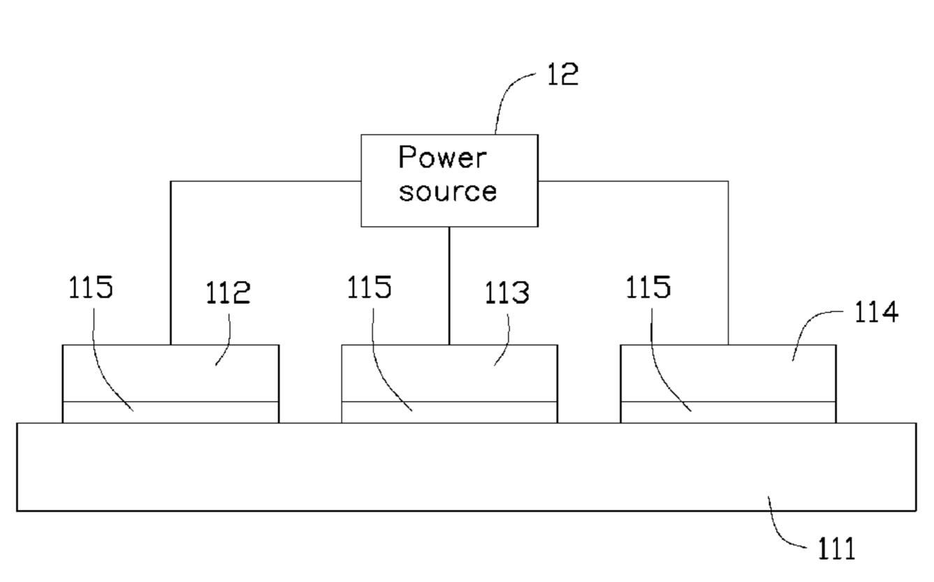
Providing a substrate having a red light LED, a green light LED and a blue light LED arranged thereon Providing a power source to supply power for the red light LED, the green light LED and the blue light LED Calculating a temperature difference  $\Delta T1$ of the red light LED, a temperature difference  $\Delta T2$  of the green light LED, and a temperature difference  $\Delta T3$  of the blue light LED Adjusting input currents of the light LED,
