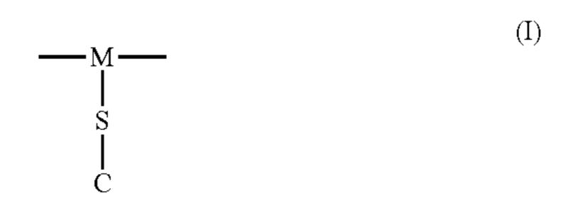
wherein M is an atom of the polymer skeleton, S is a spacer and C is a crystallizable group.
