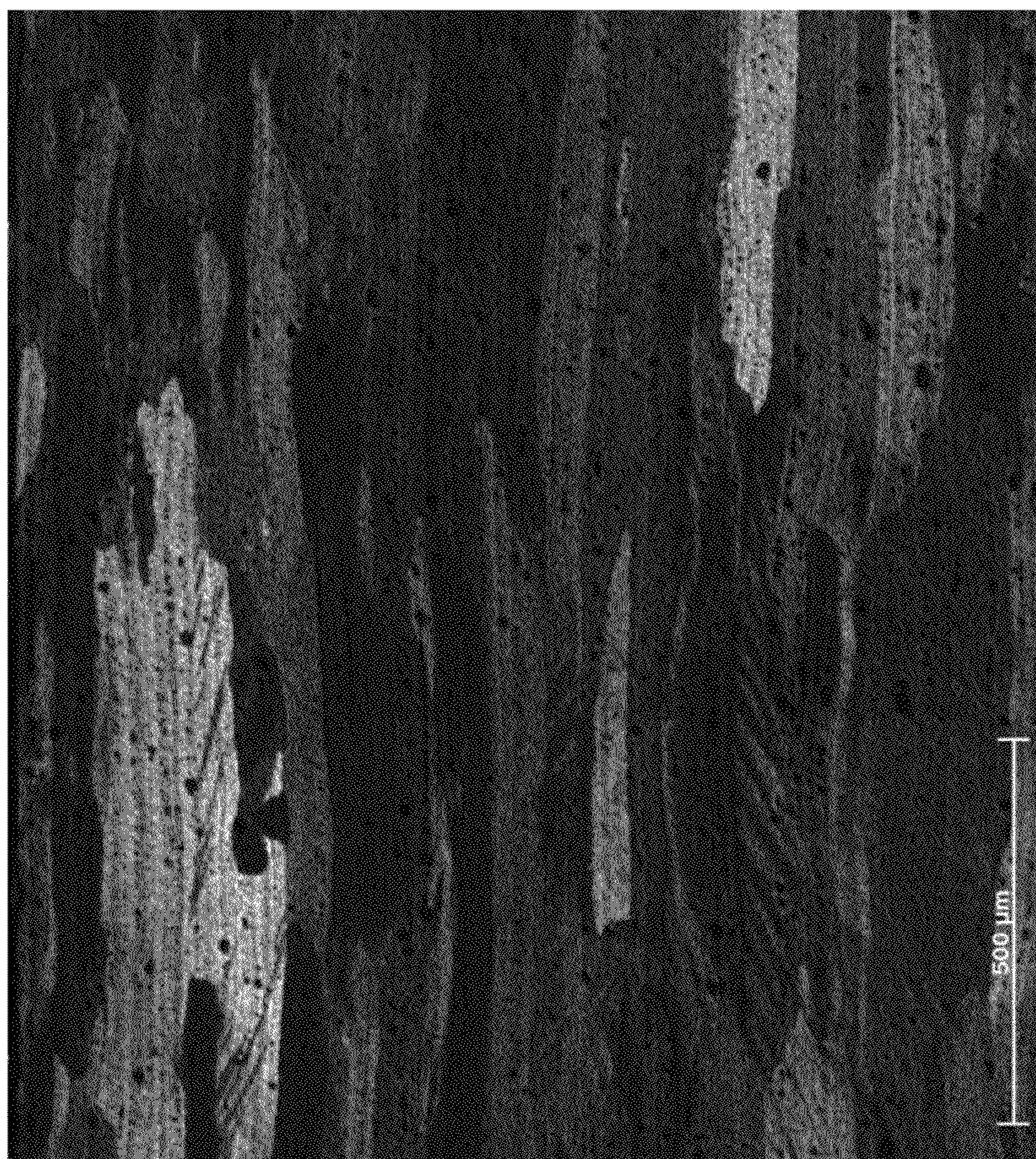
6xxx+Cu+Zn Aluminum Alloy – 35% CW
