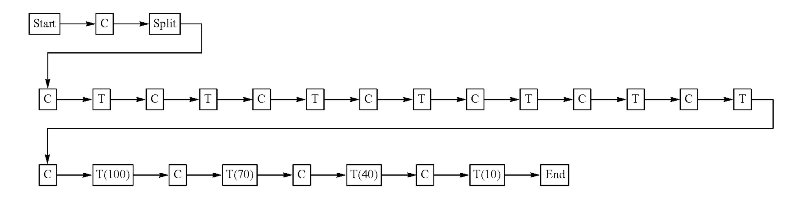
where C=conditioning cycle, T=test cycle, (x)=blade tip <sup>40</sup> speed during the test cycle (mm/s), and Split=splitting of vessel to provide precise volume of powder for measurement. The powder mass was automatically recalculated after splitting. The blade tip speed was 100 mm/s where not defined in brackets (during Rep sequence).
