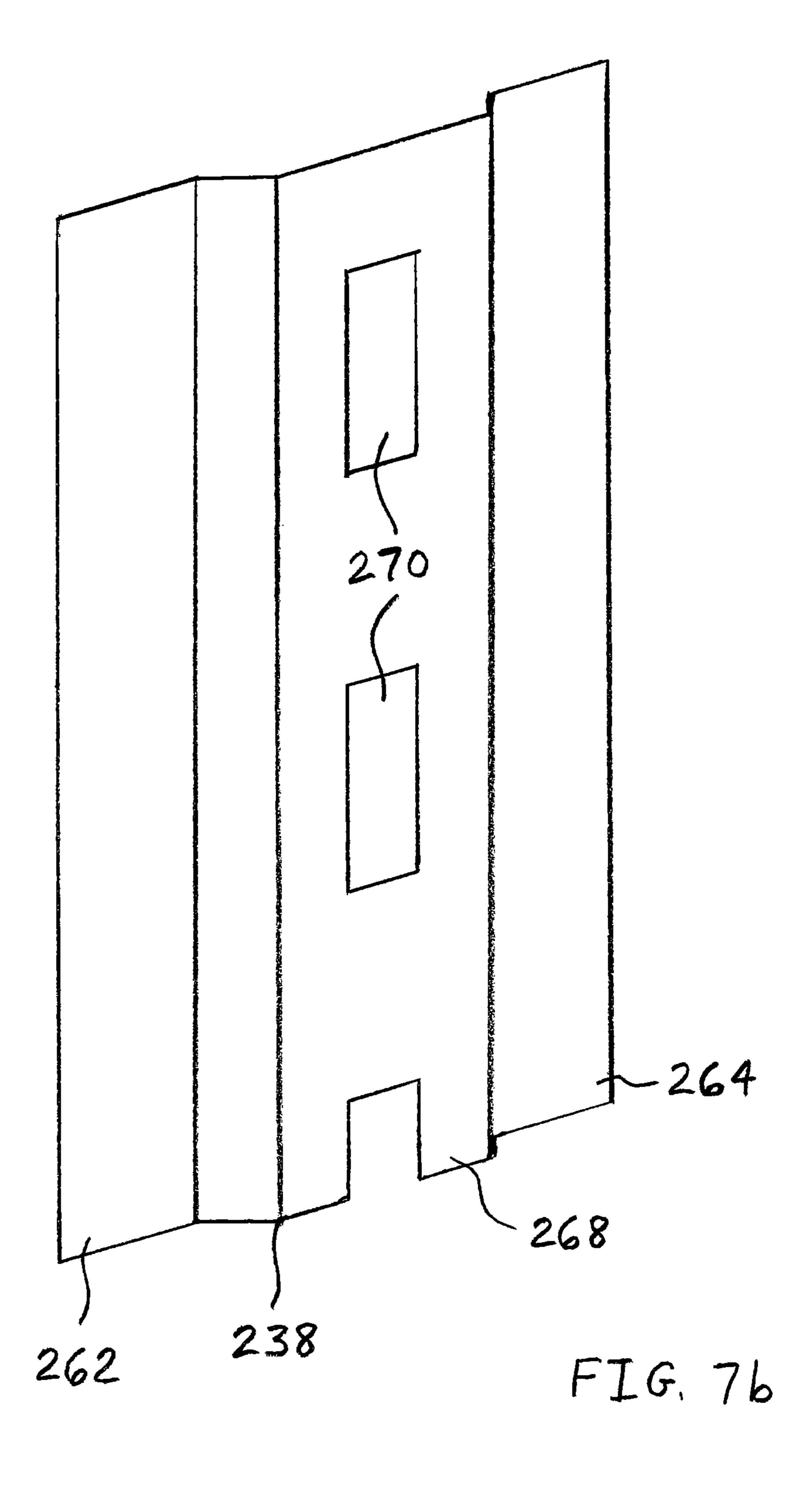
provide a plurality of upstanding panels, each panel including two opposing flanges, the flanges being disposed on opposing lateral edges of the panel (802)
