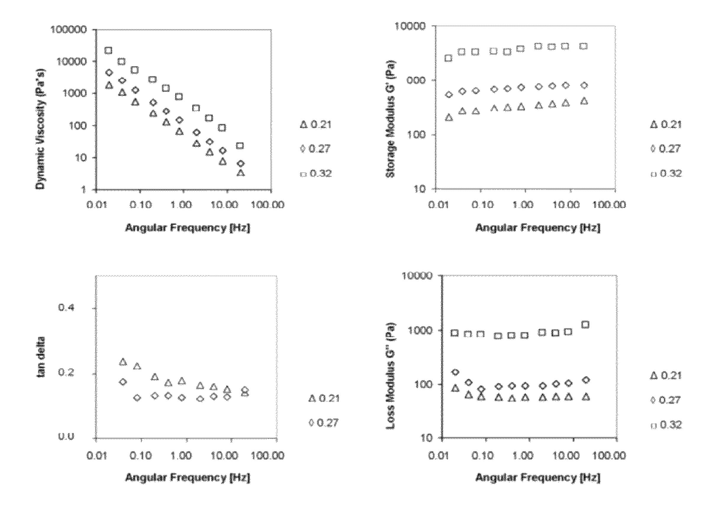
Fig. 1 Dynamic viscosity η\*, storage modulus G' and loss modulus G' and loss factor tan δ of hydrogels on the basis of Indulin, oxidized with hydrogen peroxide/iron (II) chloride tetrahydrate, cross-linked with different quantities of poly (ethylene glycol) diglycidyl ether (0.21; 0.27; and 0.32 mmol/g Indulin).
