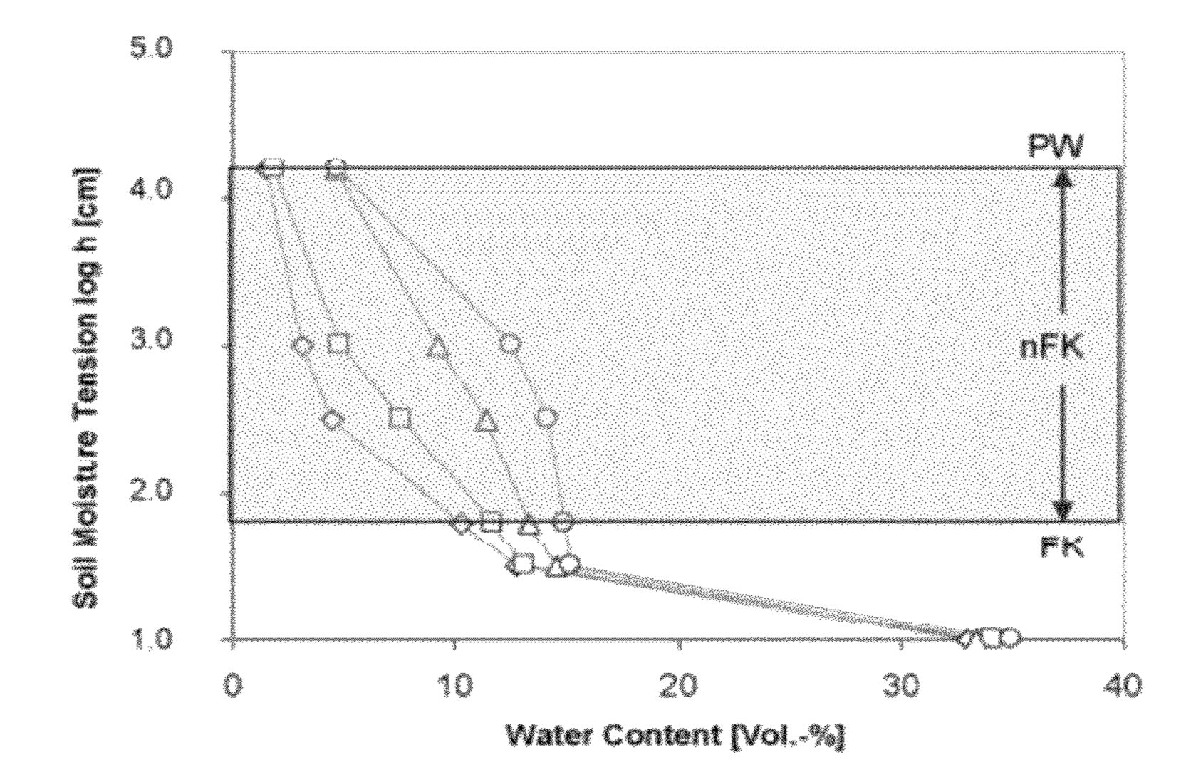
Fig. 2: Water retention curves of pure sand treated with different quantities (zero variant ♦, 0.1 % by weight □, 0.25 % by weight △, 0.5 % by weight ○) of a lignin hydrogel (variant IND ox-III-PEGG = Indulin oxidized with hydrogen peroxide/iron(II) chloride tetrahydrate crosslinked with poly (ethylene glycol) diglycidyl ether. FK = field capacity, nFK = useful field capacity; PWP = permanent wilting point.
