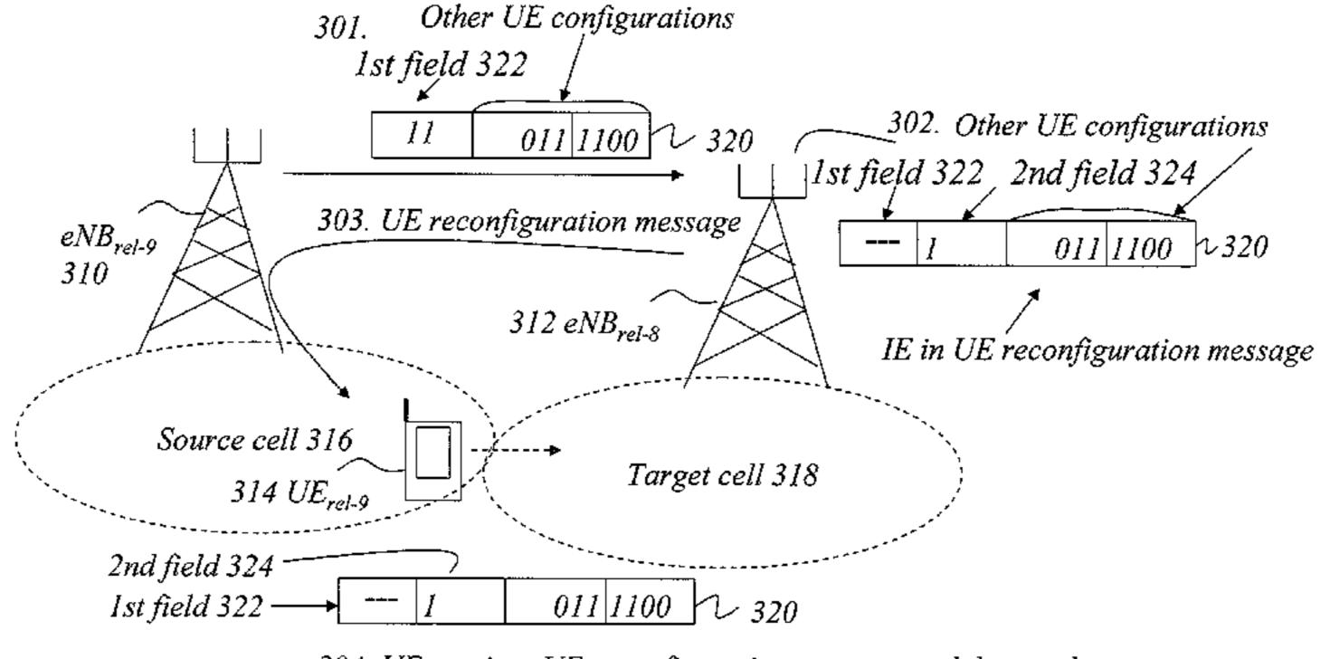
304. UE receives UE reconfiguration message and detects the 2nd field which indicates the behaviour of the UE when the 1st field is missing.
