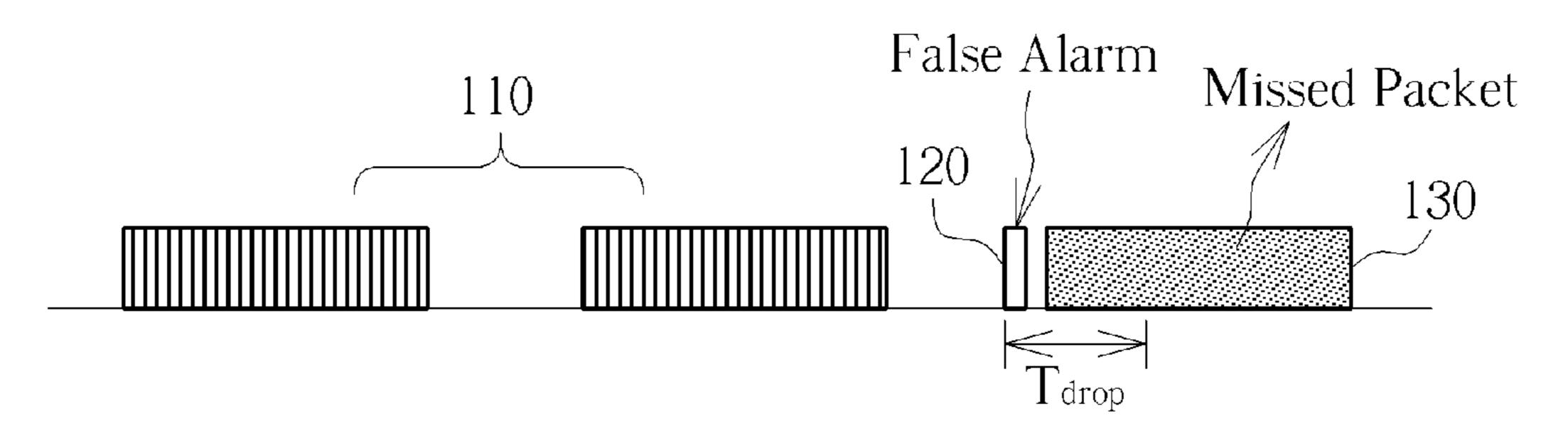
Necessary time for dropping false packet
